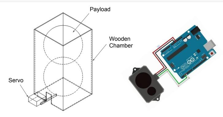
Isometric view of payload release mechanism.
