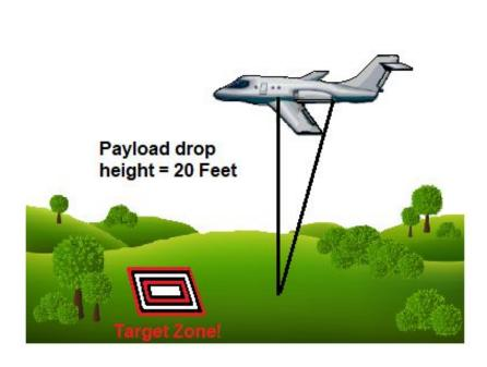
The Lidar sensor will trigger the servo to release the payload when it senses that the aircraft is lowered to 20 feet above the ground.
