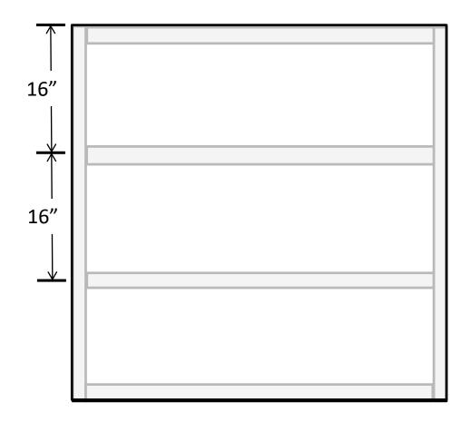
Assemble 1" x 2" structure and the 5mm x 4' x 4' Luan Panel as shown above using glue and screws as required. Memory's The Thing Sheet A Professional Mission
