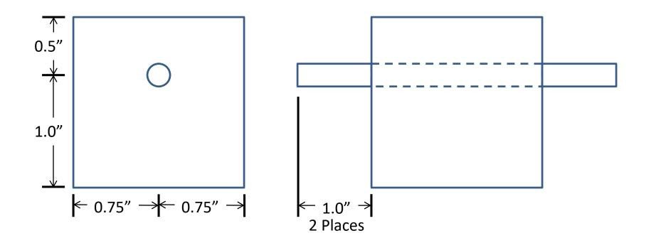
Cut (4) blocks 1.5" x 1.5". Drill and Install 5/16" dowels as shown above.
