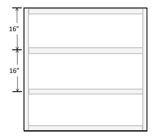
Assemble 1" x 2" structure and the 5mm x 4' x 4' Luan Panel as shown above using glue and screws as required.
