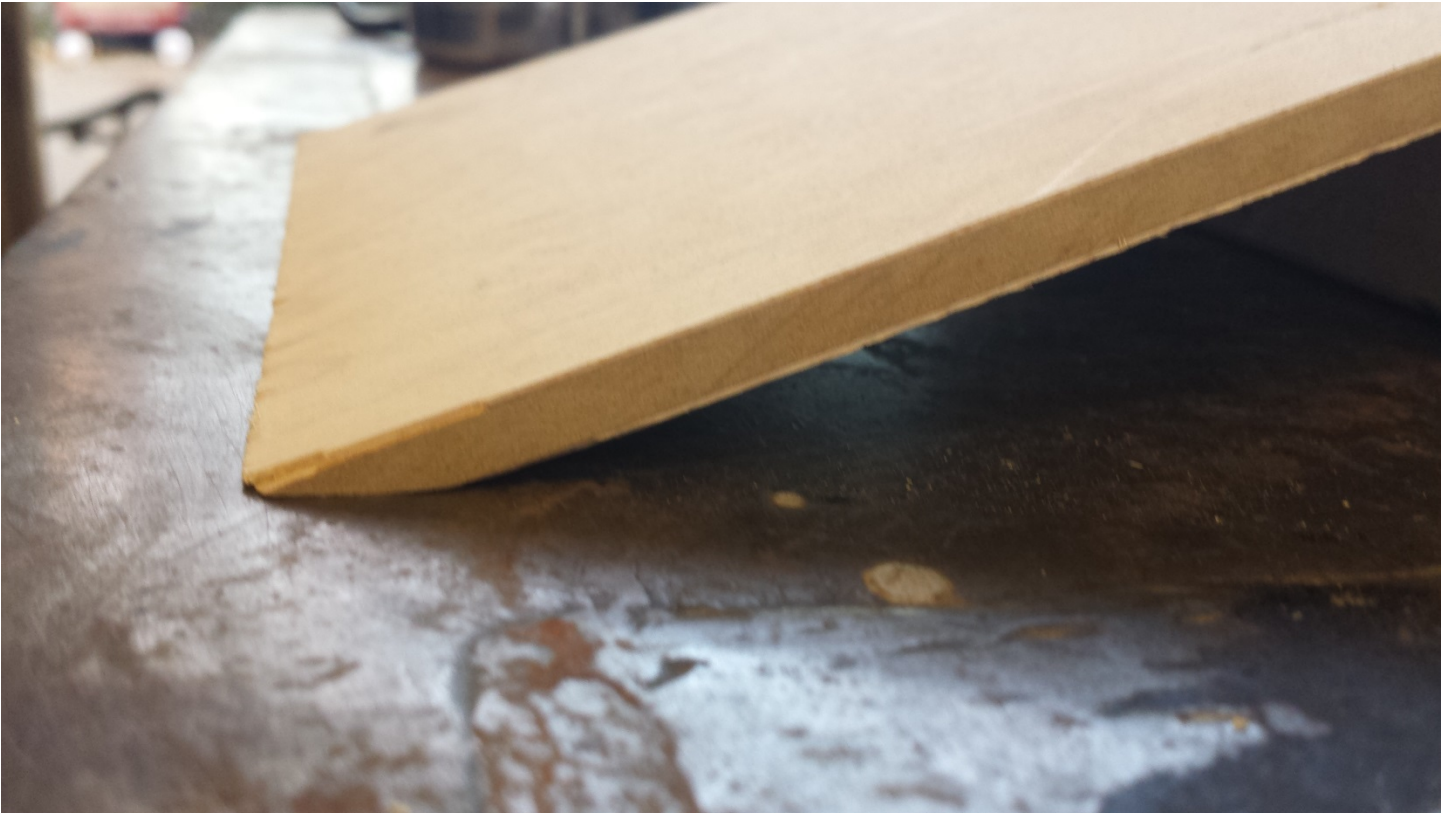
Figure 1 Tapered Bottom Edge of Ramp Incline
