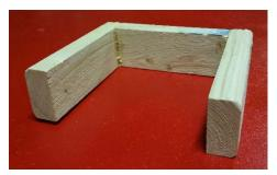
The corral was made from two 4  $\frac{1}{2}$ " and one 4" offcuts from the 1"x2" furr strip. The pieces were glued and screwed to form and a square horseshoe shape.
