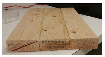
The ramps were constructed from a single two-by-four stud. The wood was cut into six 15" pieces and each ramp was made from three pieces that are glued together. Each of the four ends were cut at an angle to from the top corner to the diagonally opposite corner to create a 4" wide base at the top.
