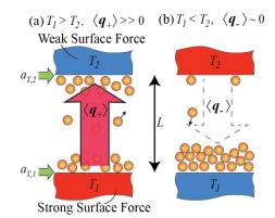
Condensable-gas-filled nano-gap with two surface force coatings acting as a thermal rectifier. (a)  $T_1 > T_2$  for  $\langle q_+ \rangle >> 0$ , and (b)  $T_1 < T_2$  for  $\langle q_- \rangle \sim 0$  due to different thermal resistance in different temperature gradient directions.
