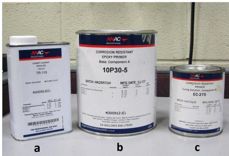
**Figure 3:** Paint used for making nanocomposite coatings: a) Thinner or Exempt Solvent Reducer P/N TR-115, (b) Epoxy Primer P/N 10P30-5, and (c) Hardener or Curing solution P/N EC-275.
