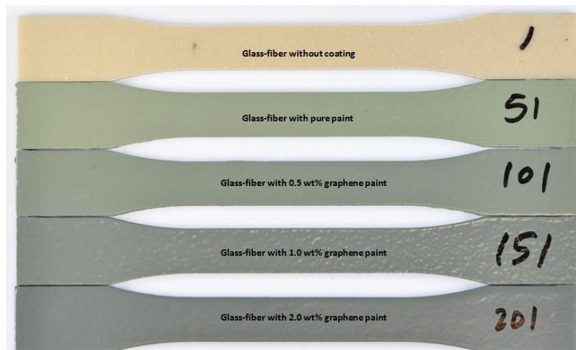
**Figure 20:** The coated and uncoated composite specimens that were used in the tensile testing.
