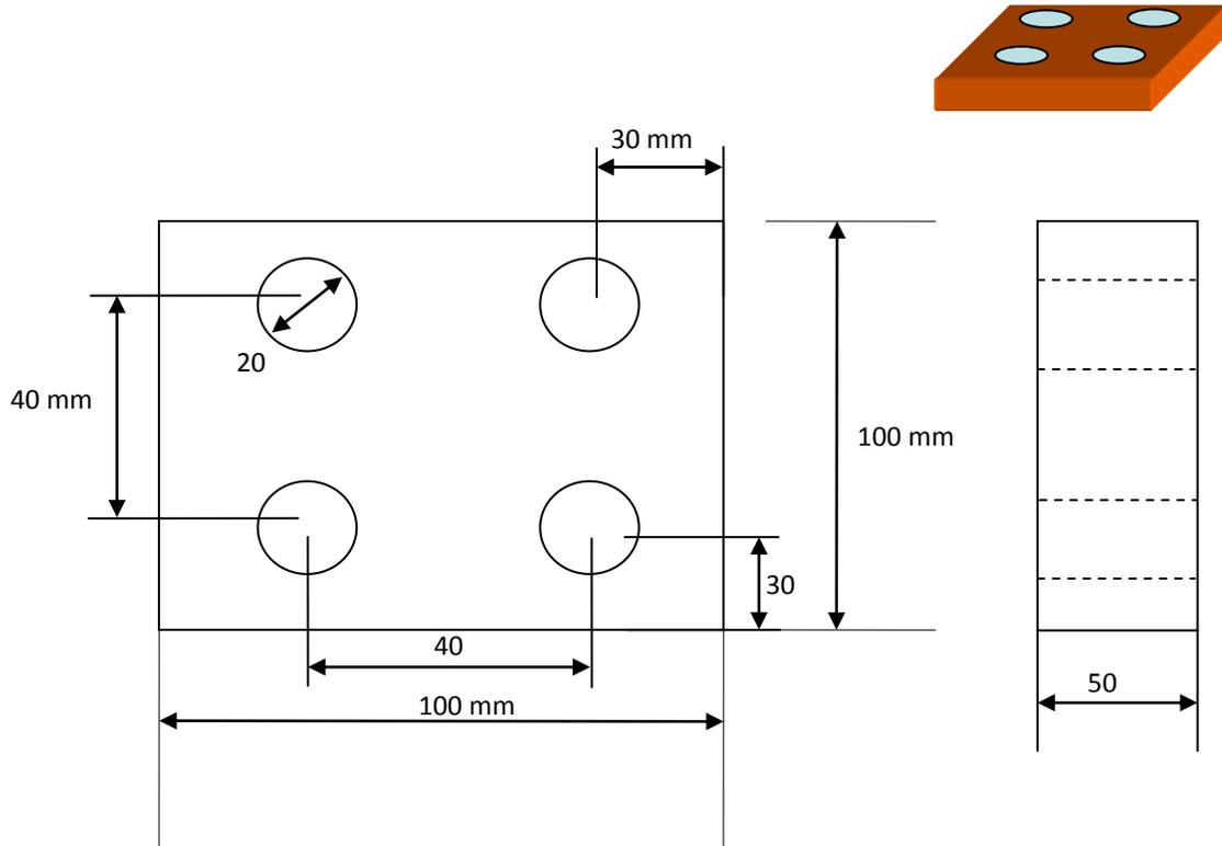
**Figure MR 1.9.** Dimensions of the Work piece
