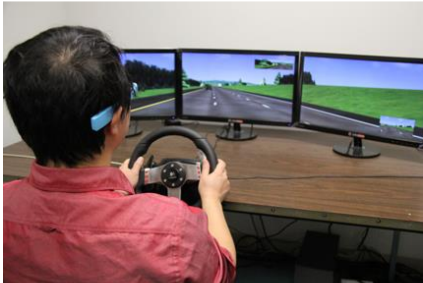
Figure 1. The HyperDrive advanced driving simulator setup. (Demo driver is wearing Google Glass while driving)
