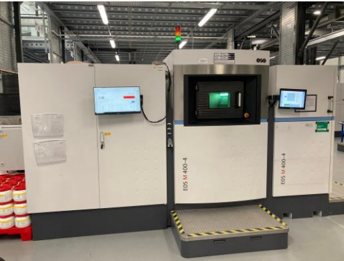
Multi-laser 400W systems; 12 Ni & 1 Ti
