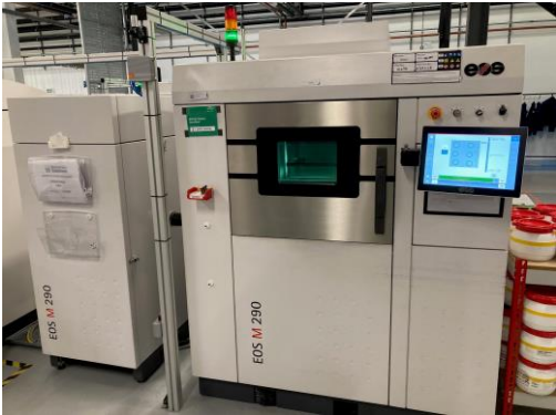
Single laser 400W system; 6 Ni, 1 Al
