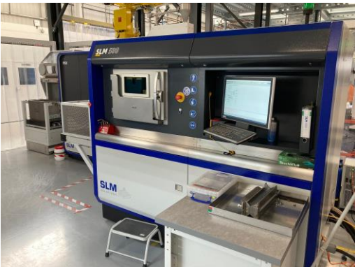
Multi-laser 700W system dedicated to Al alloys
