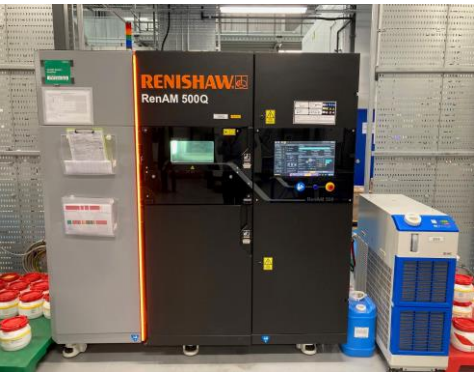
Multi-laser 500W system dedicated to Ni alloys
