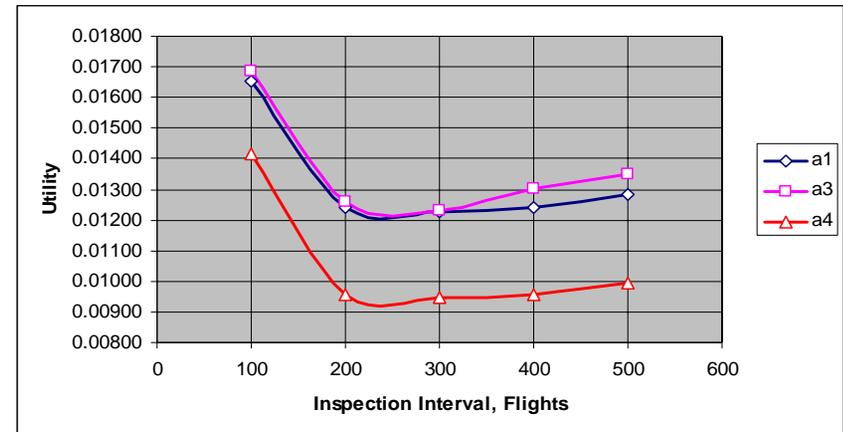
**For large damage that will be repaired within a few flights: key factor is repair quality**
