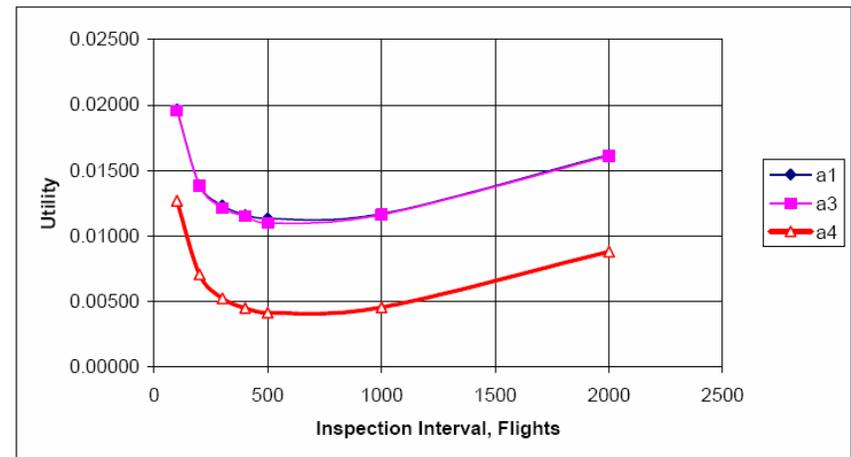
For small damages that will remain undetected for a long time: Key factors are repair quality + POD
