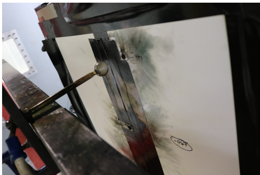
Figure 60: Arc Entry Test -Z3C5700-67-Installation-Zone 3-TP1-Post-Test
