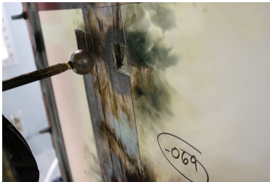
Figure 43: Arc Entry Test -Z3C5700-69-Installation-Zone 3-TP1-Post-Test
