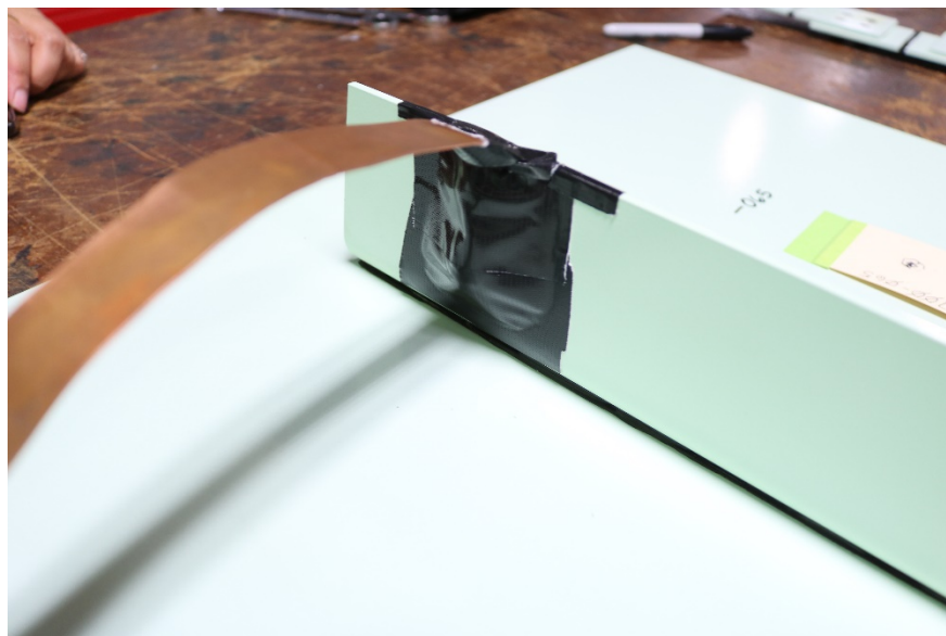
Figure 27: Arc Entry Test -General Test Setup-L bracket Bonding-3
