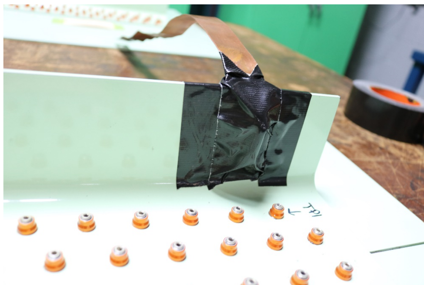
Figure 28: Arc Entry Test -General Test Setup-L bracket Bonding-4
