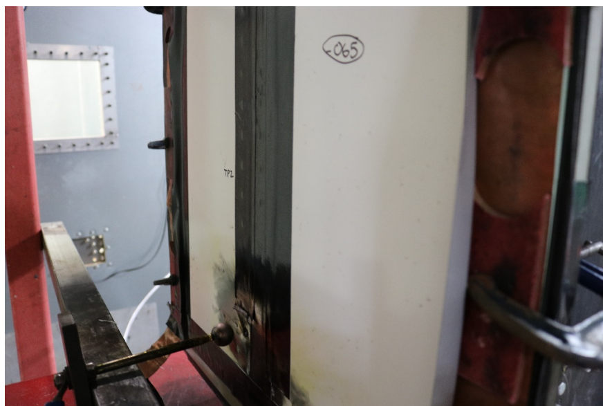
Figure 30: Arc Entry Test -Z3C5700-65-Installation-Zone 3-TP3-Post-Test
