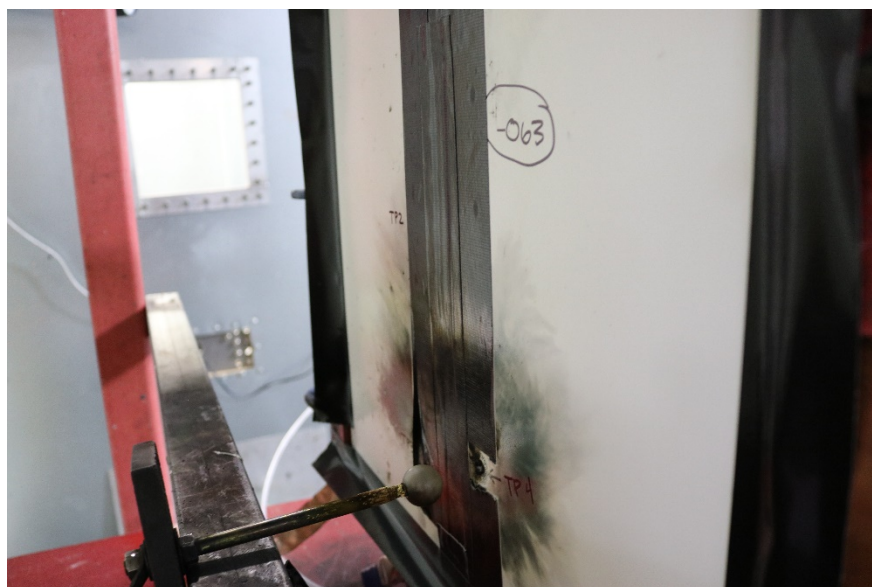
Figure 20: Arc Entry Test -Z3C5700-63-Installation-Zone 3-TP4-Post-Test
