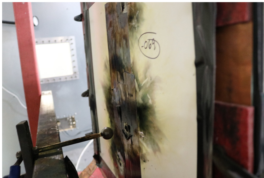
Figure 45: Arc Entry Test -Z3C5700-69-Installation-Zone 3-TP4-Post-Test
