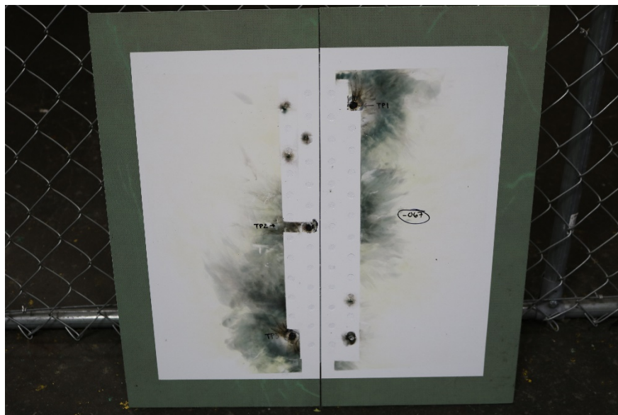
Figure 61: Arc Entry Test -Z3C5700-67-Zone 3-Post-Test-Front
