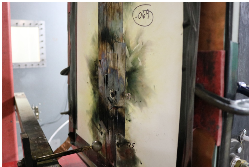
Figure 47: Arc Entry Test -Z3C5700-69-Installation-Zone 3-TP5-Post-Test
