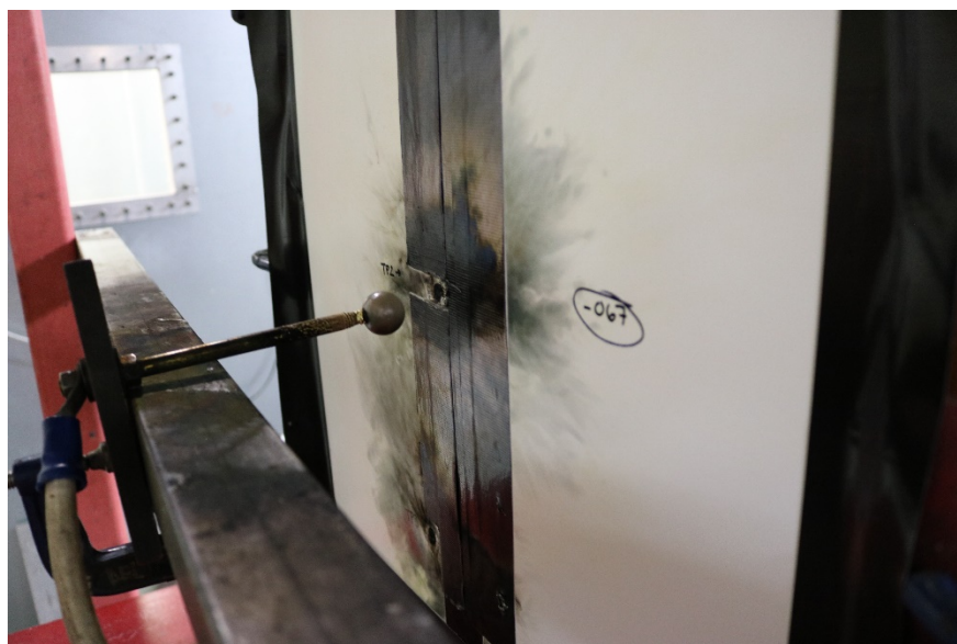
Figure 58: Arc Entry Test -Z3C5700-67-Installation-Zone 3-TP2-Post-Test
