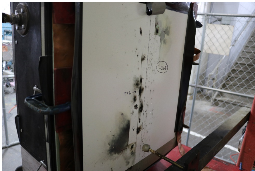
Figure 17: Arc Entry Test -Z3C5700-63-Installation-Zone 3-TP3-Post-Test-2
