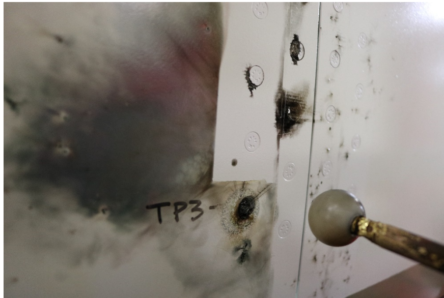
Figure 6: Sample Photo of Exterior Side Damage to Fastener
