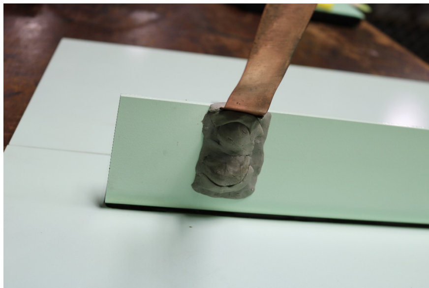
Figure 35: Arc Entry Test -General Test Setup-L bracket Bonding-5
