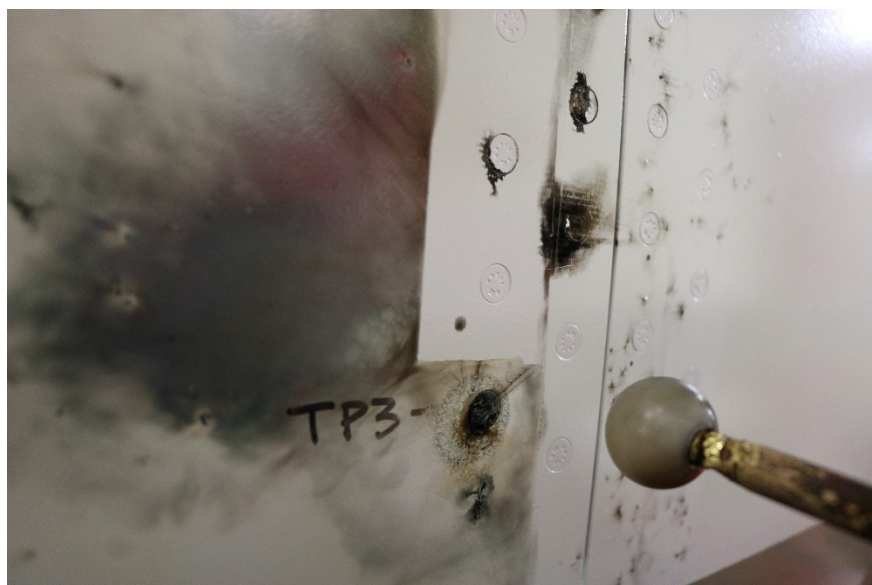
Figure 18: Arc Entry Test -Z3C5700-63-Installation-Zone 3-TP3-Post-Test-3
