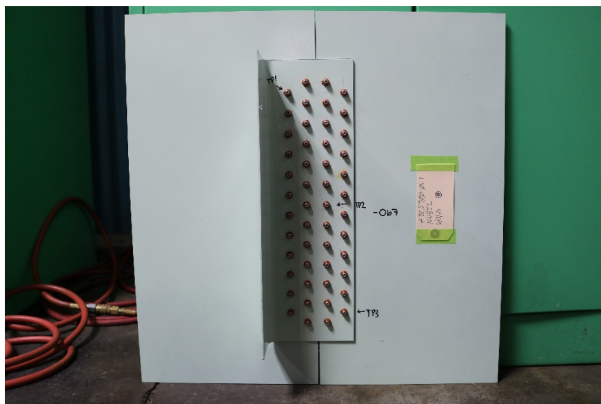
Figure 8: Arc Entry Test -Z3C5700-67-Check In-Pre-Test-Back-Incorrect Fastener
