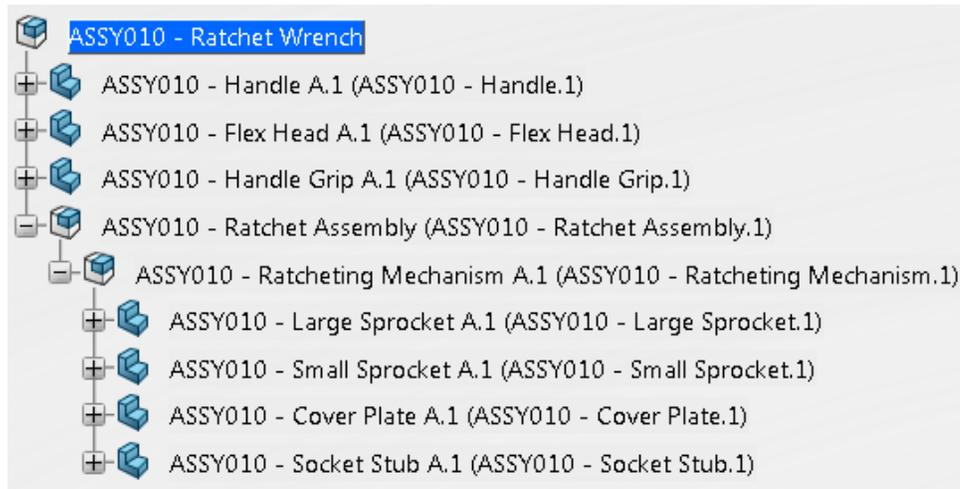
The Flex Head part should be part of the Ratchet Assembly. It will be added to the new subassembly.
