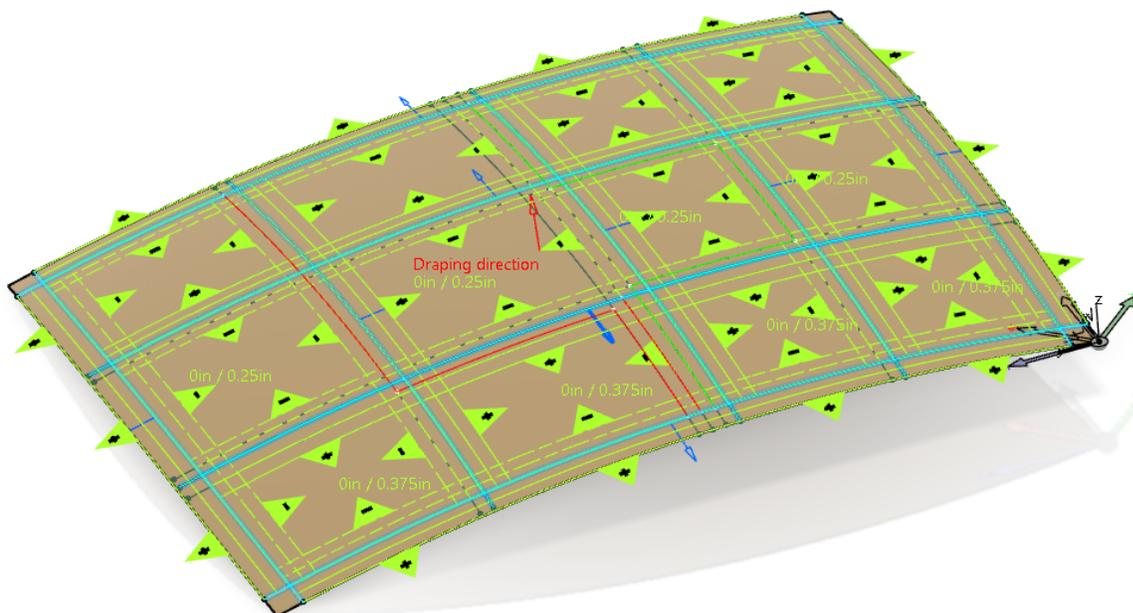
Change the ramp definition for *Parallel.6* to use the *0in / 0.375in* ramp definition in both directions. You can simply select the *0in / 0.375in* ramp definition from the drop down to reuse the one you just created.
