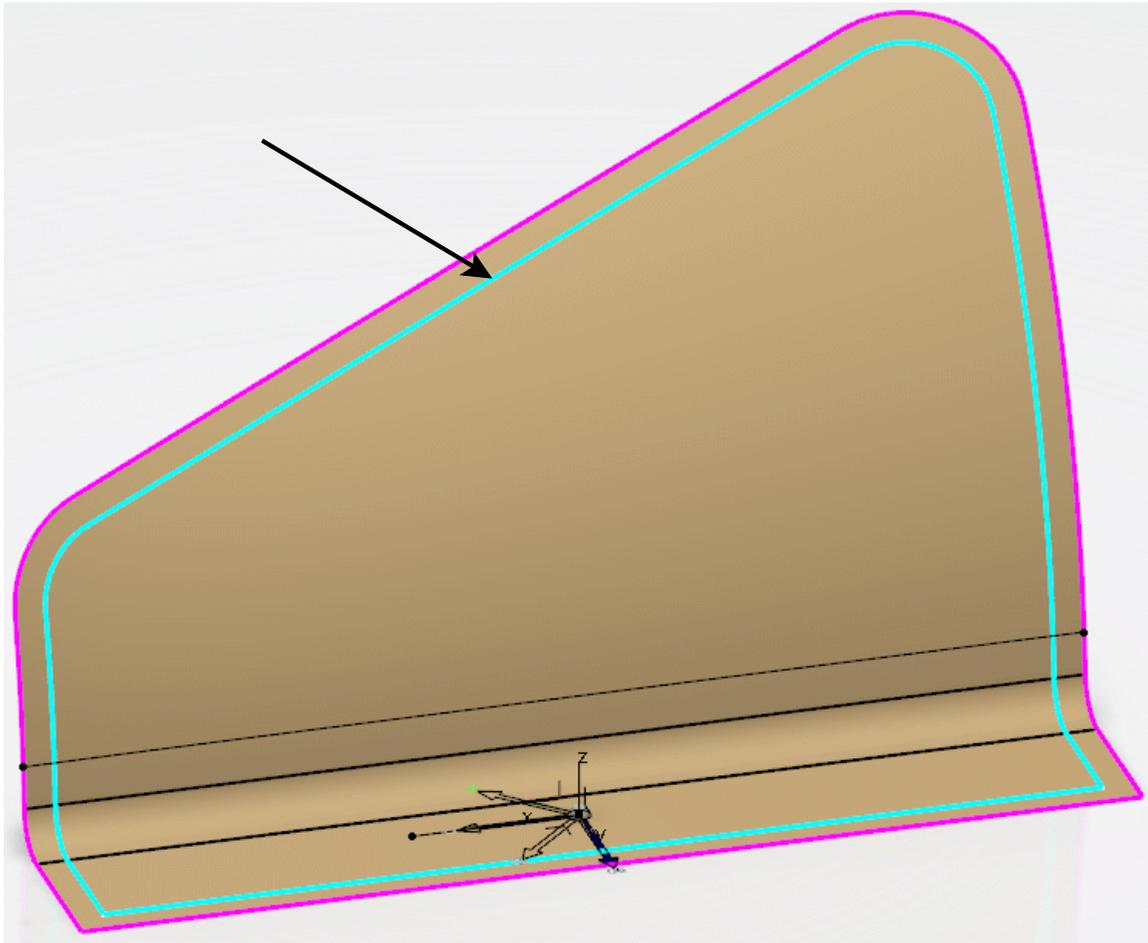
Select the *Attributes* tab and set the *Material* to be *Carbon Fiber Cloth* and the *Direction* to be **0**. This will define the first ply.
