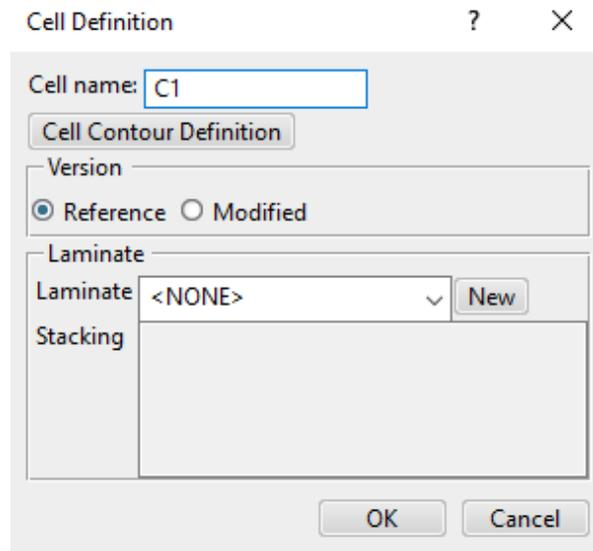
Change the *Cell name* to be **9 Ply Zone** and select the *New* button for the *Laminate* option. The *Laminate* window appears.
