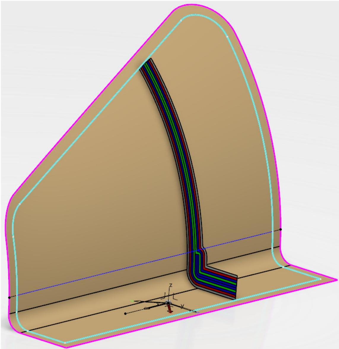
Notice the laminate is completely symmetric. This provides an easy method for creating a very simple layup of plies without having to use an advanced design method. Keep in mind that if you wanted to have any staggering in the plies that are dropped off, you would have to create wireframe curves to be able to manually select the shape of each ply. For this reason, this method only works well for pretty simple laminates.
