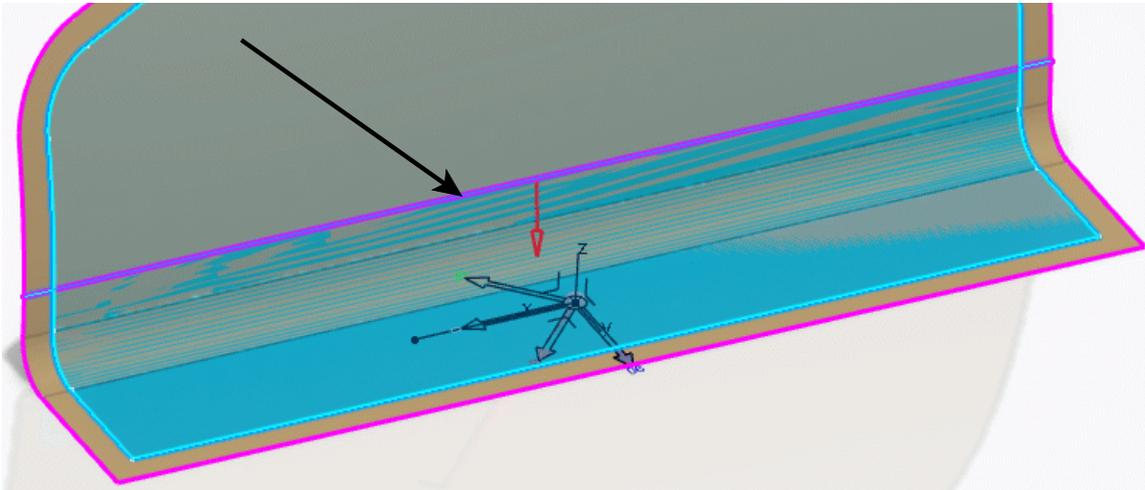
Be sure the arrow is pointing towards the lower portion of the surface and select **OK**. This specifies the lower side of the ply will be kept.
