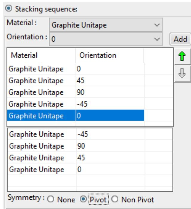
**Select *OK*.** This defines the thickness law as well as the actual order of the stacking for constant area. The *Cell Definition* should appear as shown.
