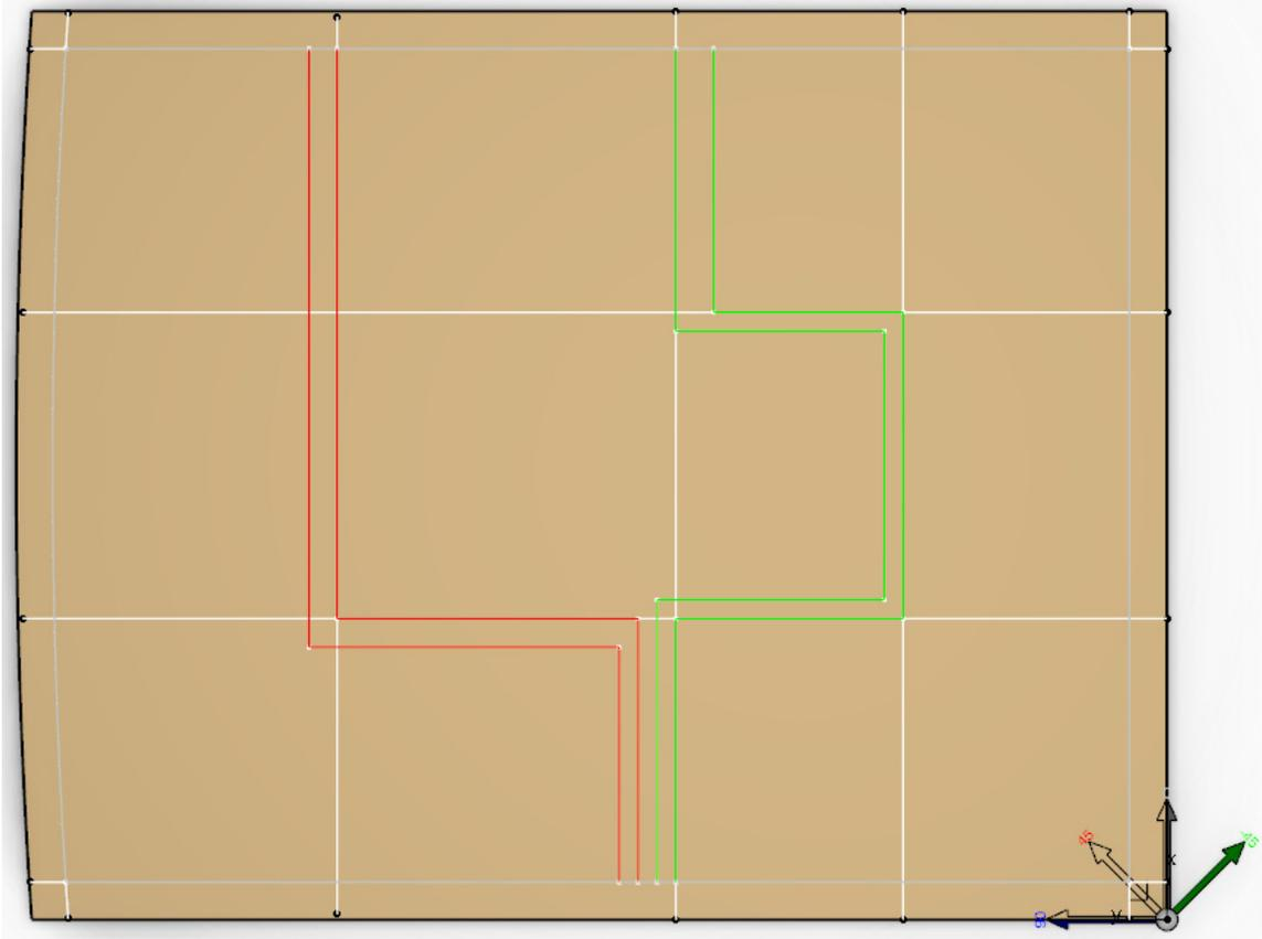
**Explode the plies with the Shell Constant Offset option and a Scale of 10.**
