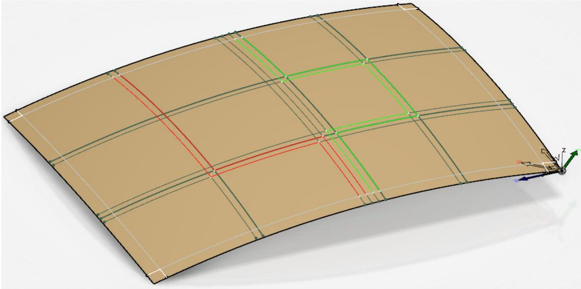
Most of the drop offs are correct, but a few need to be modified to have the correct staggering. Fortunately, the original grid panel definition can be modified and the plies will automatically update.
