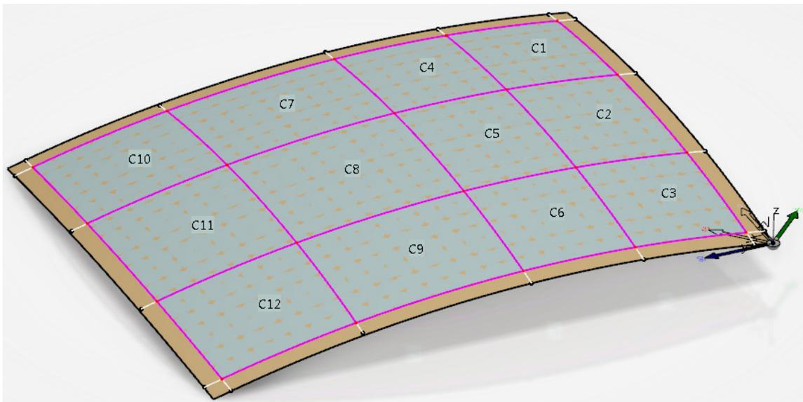
First, the cells that will be a common thickness will be merged together to simplify the panel definition. Keep in mind this is typically not recommended. Leaving the cells in their default definition will yield more robustness to the design.
