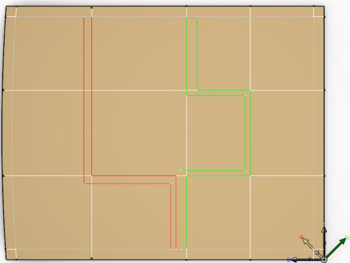
**Select all of the curves from the display as shown to define the first reference element group.** The curves could be split into multiple reference element groups if necessary. In this case, only one group will be used.
