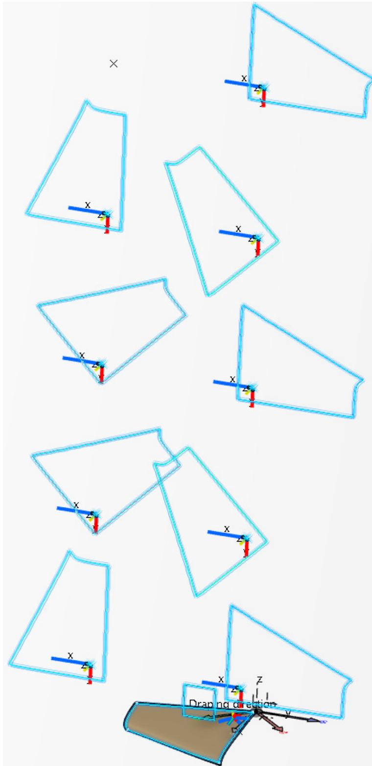
Select the *Unfold assembly* option. Set the *Continuity to Threshold* and the *Tangency threshold to 10*, turn on the *Curvature threshold* and select *OK*. The plies are positioned in a more uniform manner this time. The plies were also smoothed in tangency.
