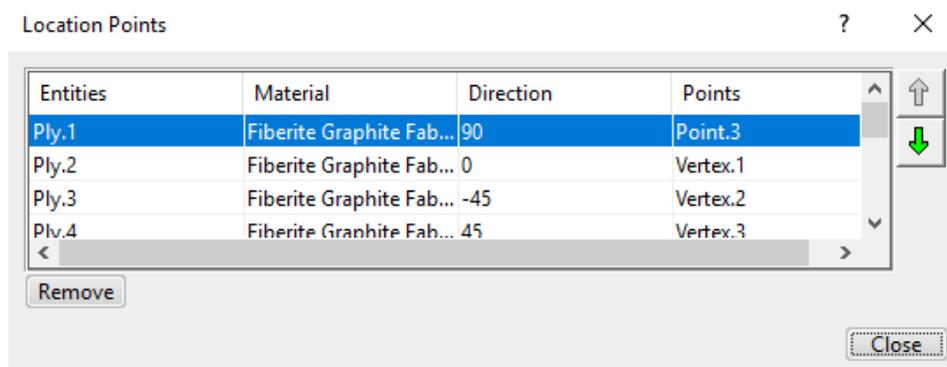
Notice all of the plies are listed and each ply was assigned a location point. You can manually specify which ply is assigned to which point from this window if you wanted to.
