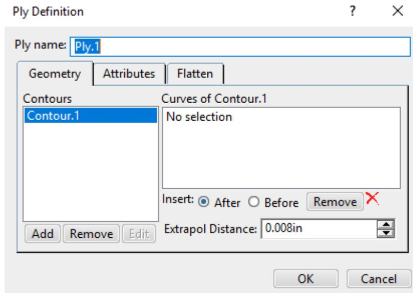
Select the curve in the display to define the contour. A green checkmark should appear in the window, specifying it is a closed contour.
