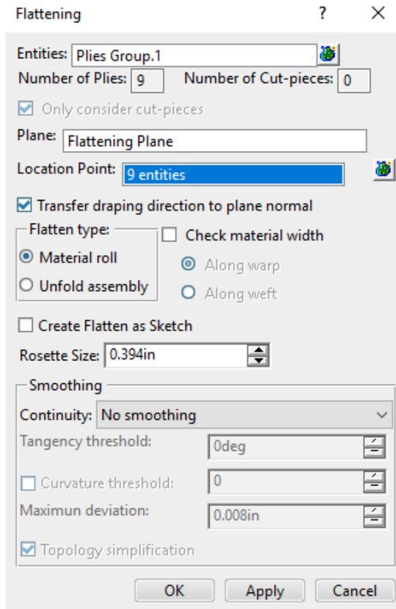
Notice there are 9 plies selected and 9 point locations as well. Selecting a pattern will automatically assign the plies or cut pieces to each point in the pattern.
