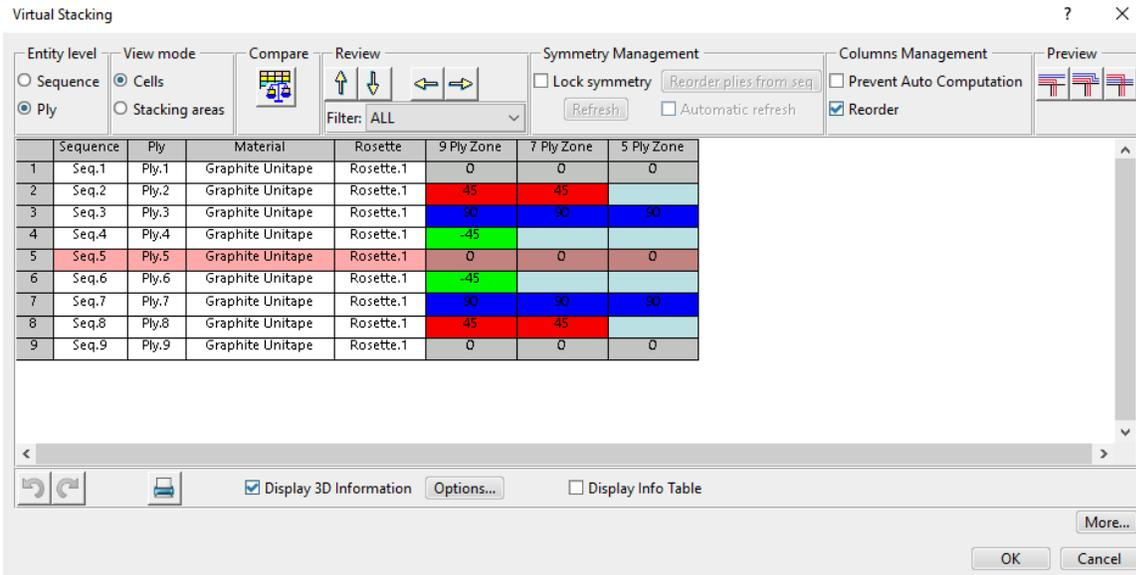
Since the stacking sequences were already defined for the cells, it is not necessary to rearrange the rows in this window. If any changes were needed, they could be made though.
