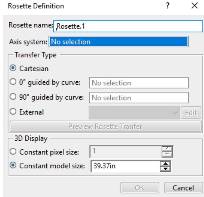
Select the axis system from the display to define the *Axis system* for the rosette. Adjust the size of the rosette and select **OK**. The rosette is created.
