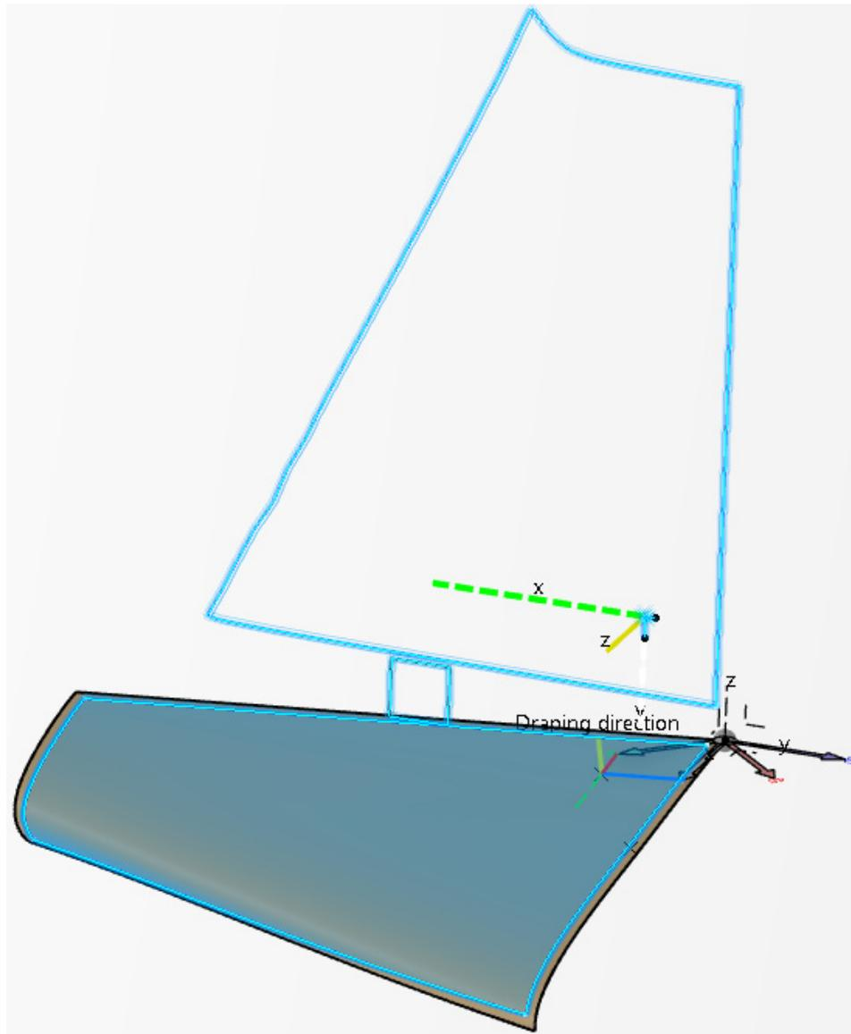
Notice the original point that was selected during the producibility operation is positioned at the specified point from the flattening operation.
