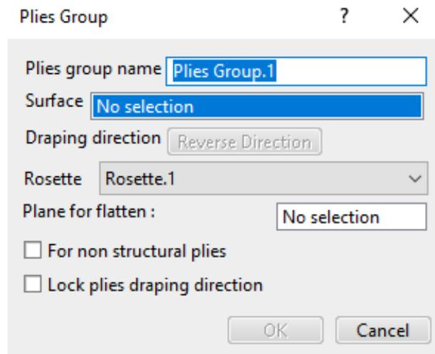
Select the surface from the display to define the *Surface* option. The draping direction should be pointing upwards.
