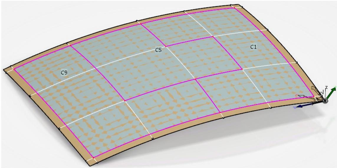
Select the cell as shown and select the *Edit* button. The name and stacking sequence for the cell will be modified.
