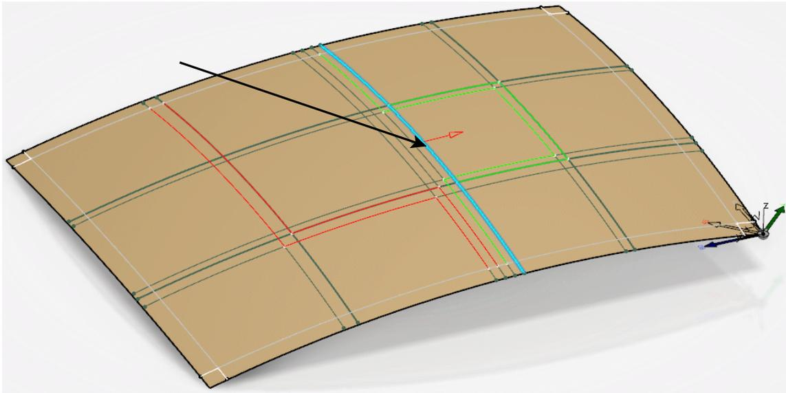
Select the **Side +** option and set the **Curves count** to be **3**. This specifies which side of the reference element and the number of curves to be created.
