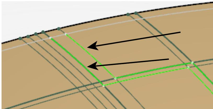
This should have all of the ply drops in the correct direction and with the correct staggering.
