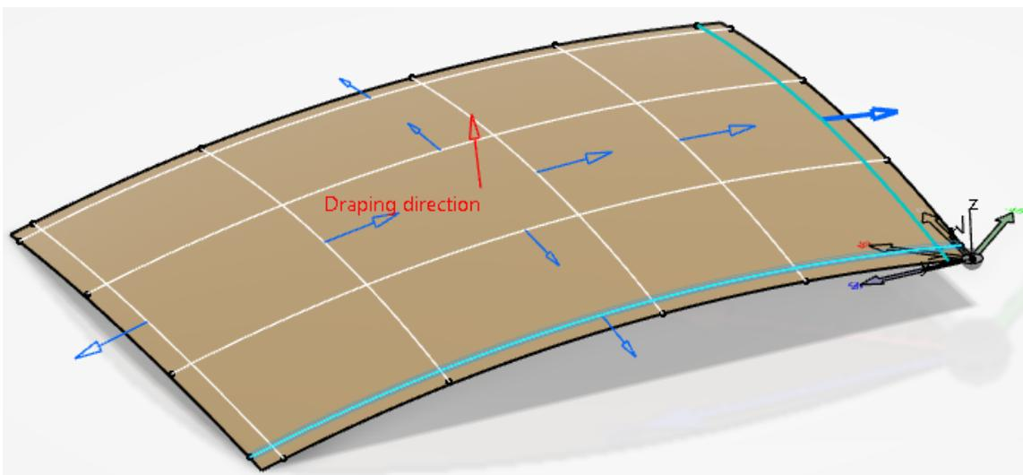
**Edit the group and create a new ramp definition with the *Offset* set to 0 and the *Step* set to 0.25 for both the positive and negative directions.** This will not work for all of the ply drops, but since it is the most common for this model, it will be used as the default. The other drops will be individually modified later. The window should appear as shown.
