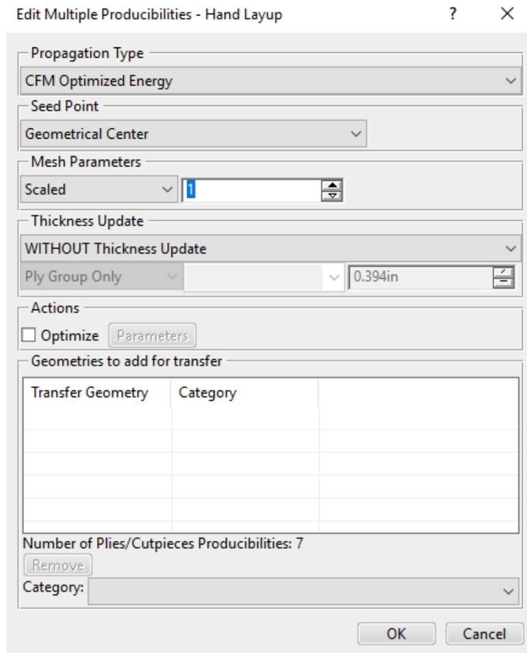
Turn on the **Optimize** option and select the **Parameters** button. The *Optimization* window appears.
