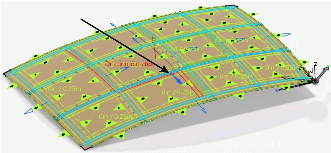
This curve should have a drop off staggering of 0.375 in the negative X direction instead of 0.25. This will be fixed now.
