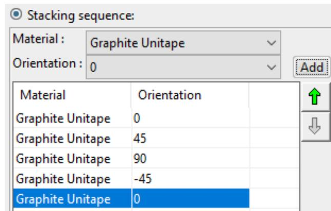
**Set the Symmetry option to be *Pivot*.** The final 0 degree ply will be the center of the laminate. The stacking should appear as shown.
