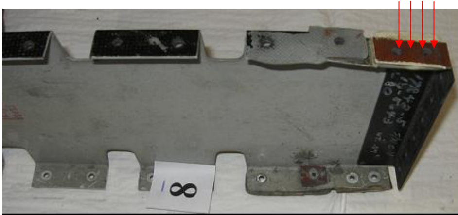
Phenolic shims used to fill gaps between skin and ribs
