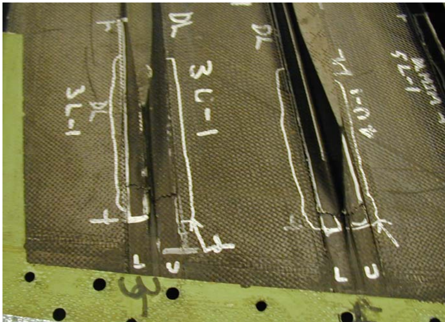
Upper skin Inboard delaminations at stringer runouts
