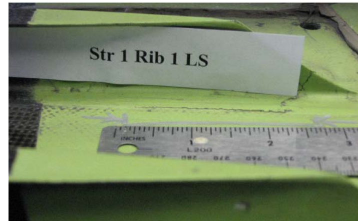
Upper skin Inboard delaminations at stringer runouts
