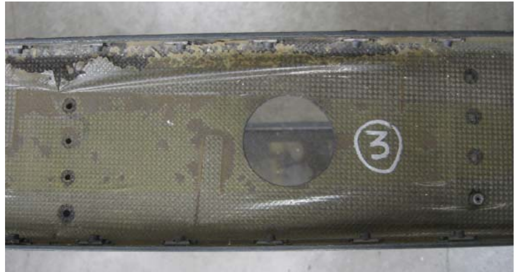
Degradation of Tedlar Moisture Barrier film
