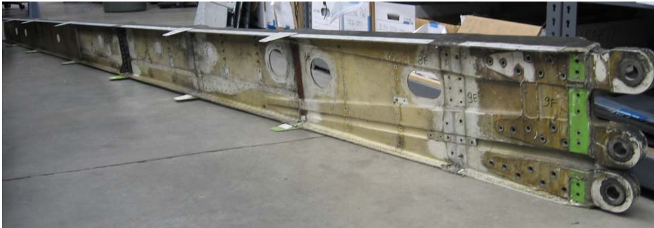
Front and Rear Spars after disassembly
