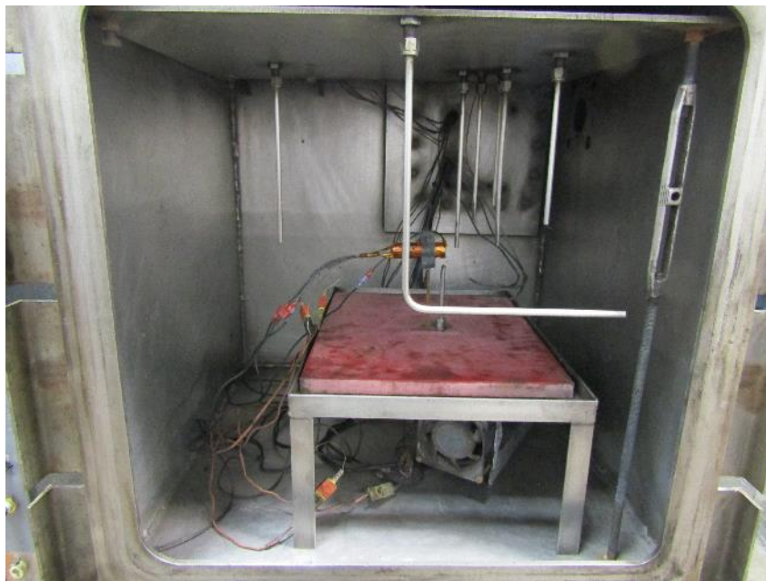
Figure 3: Thermocouple Fixture Mounted at the Top of the Thermal Runaway Chamber
