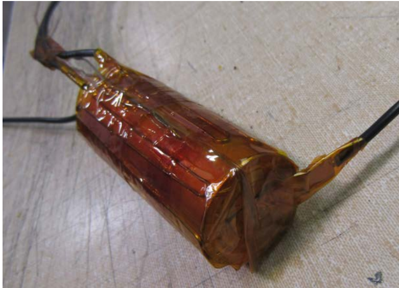
Figure 1: Nichrome Wire Resistive Heating Installation
