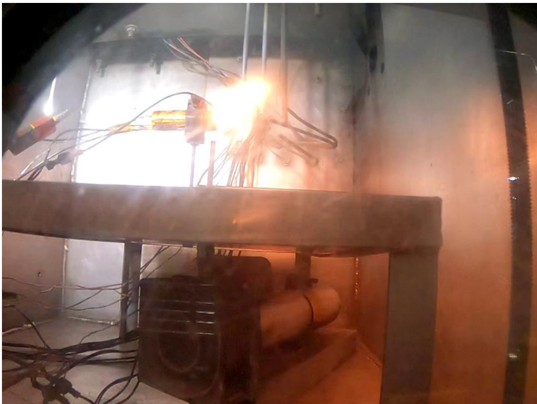
Figure 163: R5-6 Venting and Fire
