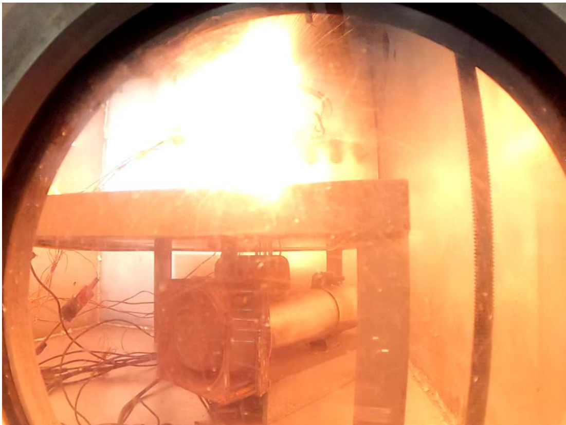
Figure 167: R5-7 Venting and Fire
