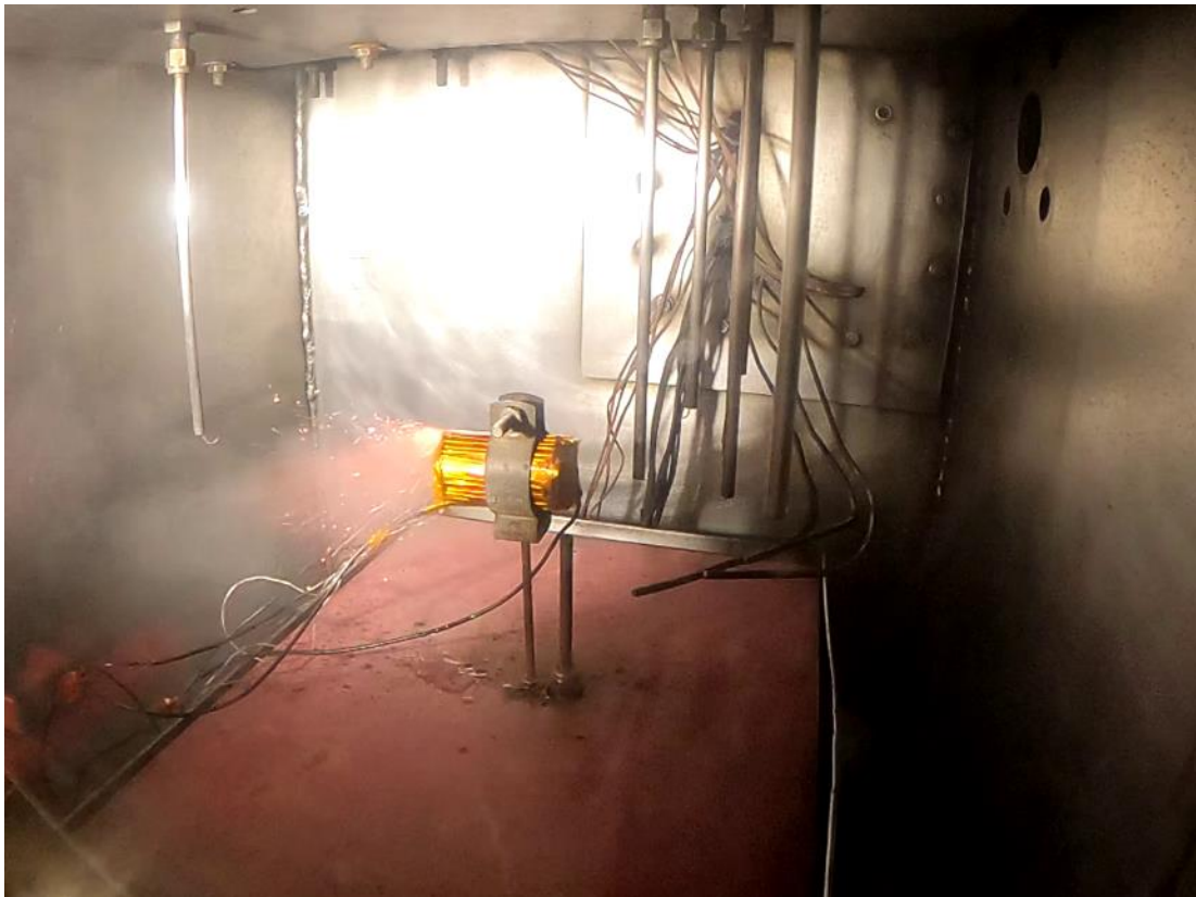
Figure 50: N2-8 Venting, Leaking, and Fire
