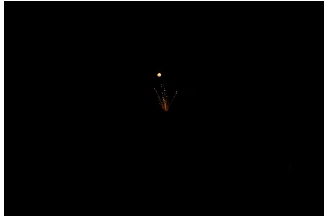
Figure 84: MN-4009-6, during test, external spark on J2
