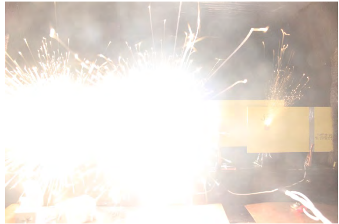
Figure 14: MN-1T03-1, during test, external sparks on all 3 joints
