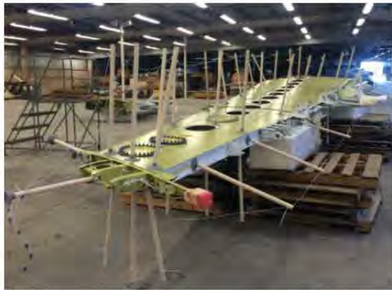
Figure 1: Retired business jet wing used as test article for this validation effort.
