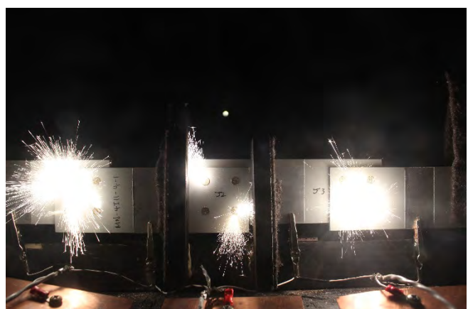
Figure 86: MN-4I11, shot 1, during test, external sparks on all 3 joints
