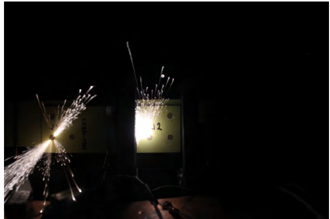
Figure 72: MN-4I03-1, during test, external sparks on J1 & J2
