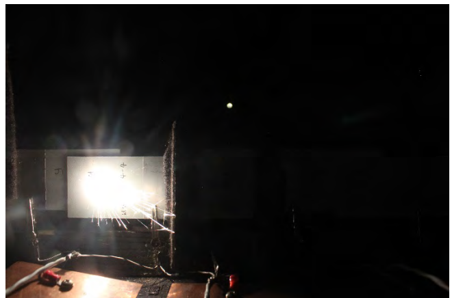
Figure 40: MN-1I11-4, during test, external spark on J1, internal spark on J3
