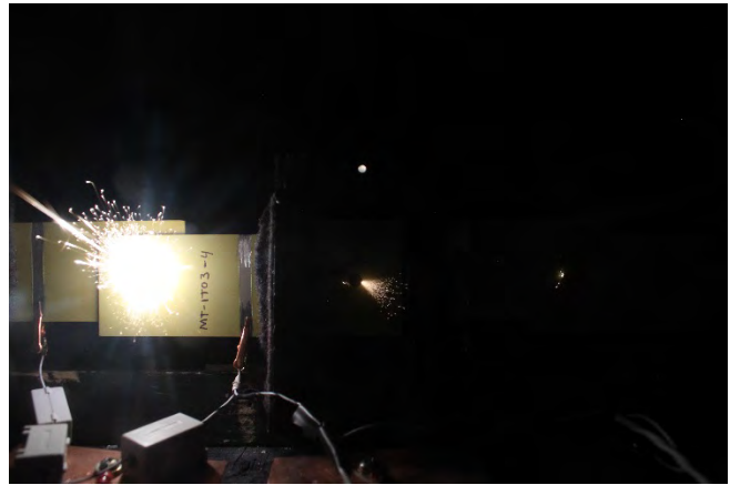
Figure 20: MN-1T03-4, during test, external sparks on all 3 joints
