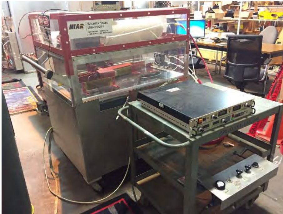
Figure 8: Front View of 25.981 Lightning Generator
