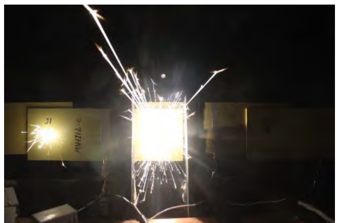
Figure 56: MN-1I12-6, during test, external sparks on J1 & J2
