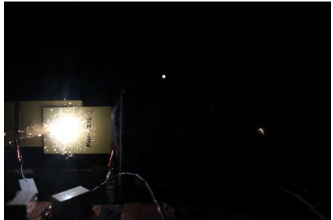
Figure 8: MN-1I12-2, during test, external sparks on J1 & J3
