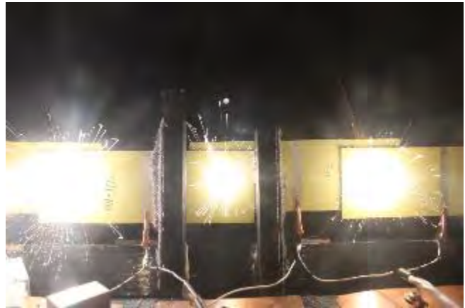
Figure 46: MN-1I12-1, shot 1, during test, external sparks on all 3 joints
