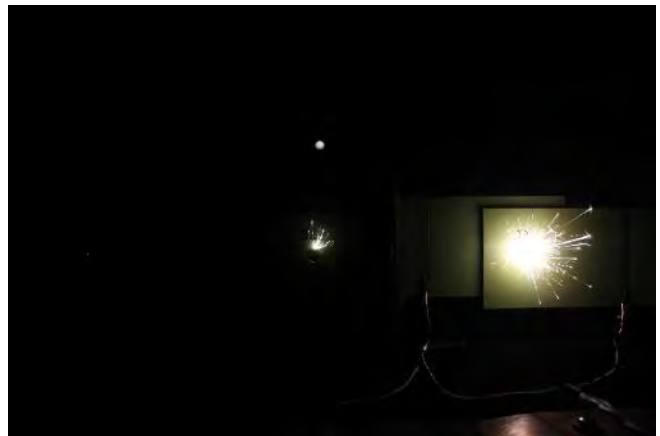
Figure 52: MN-1I12-4, during test, external sparks on all 3 joints
