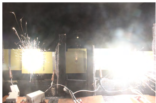
Figure 18: MN-1T03-3, during test, external sparks on all 3 joints
