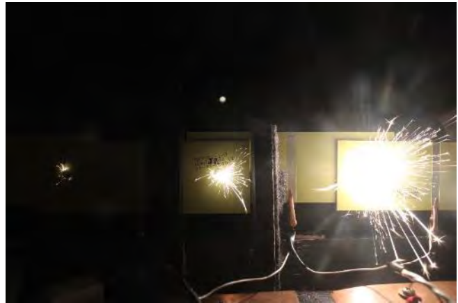
Figure 48: MN-1I12-2, during test, external sparks on all 3 joints
