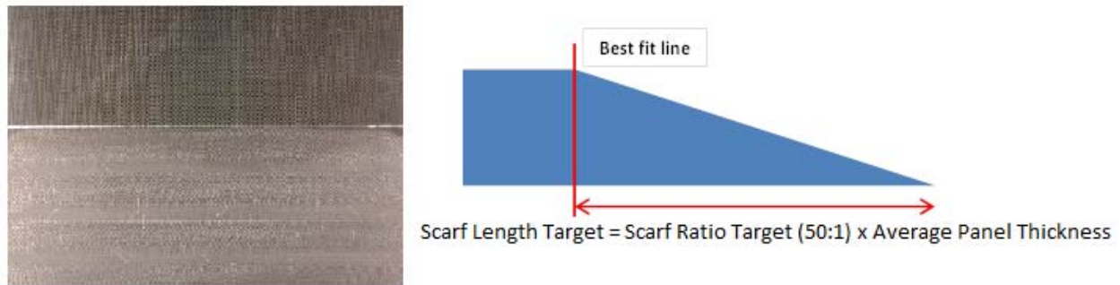
Figure 1-6: Scarf Ratio of (50:1)
