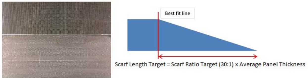
Figure 1-7: Scarf Ratio of (30:1)
