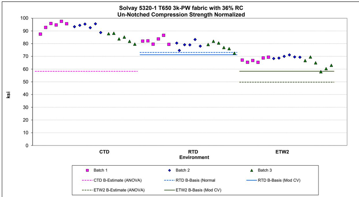
**Figure 4-1: Batch plot for UNC1 Strength**
