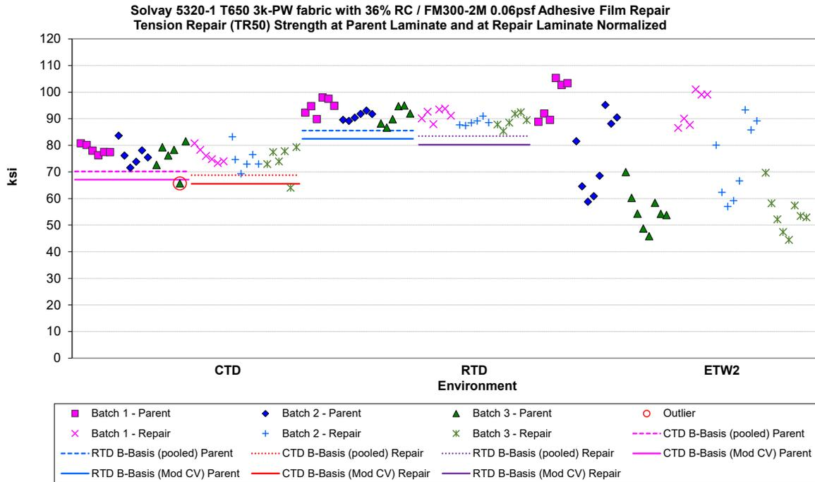
**Figure 4-8: Batch plot for TR50 Strength at Parent Laminate and Strength at Repair Laminate Normalized**
