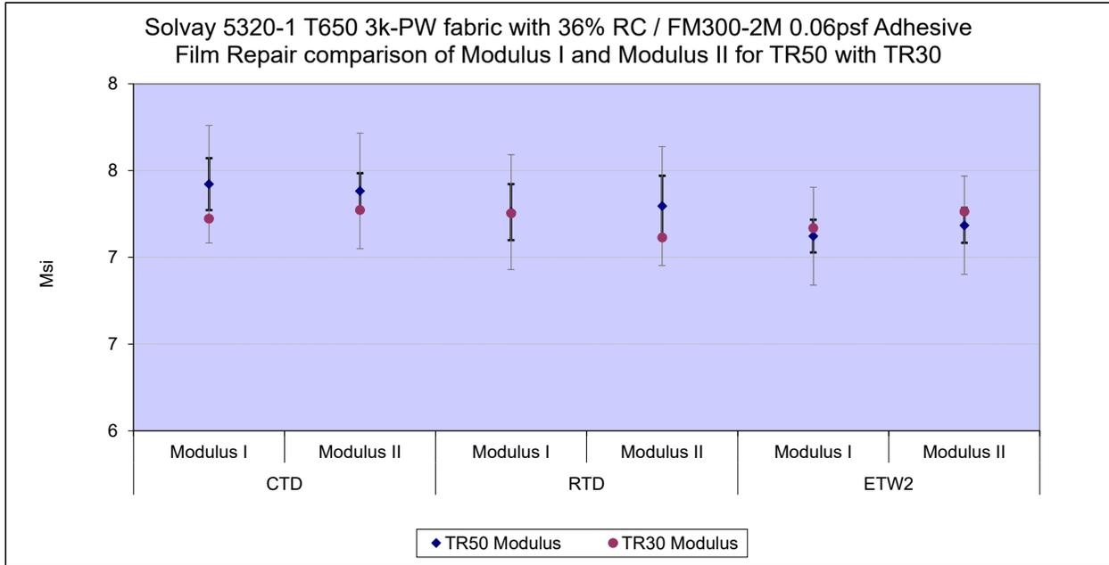
Figure 4-12: TR30 with TR50 Modulus I and Modulus II normalized means and Equivalence limits
