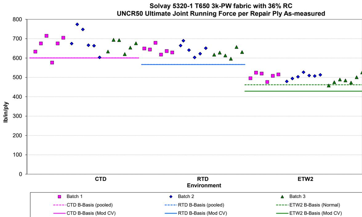
**Figure 4-3: Batch Plot for UNCR50 Ultimate Joint Running Force per Repair Ply As-measured**
