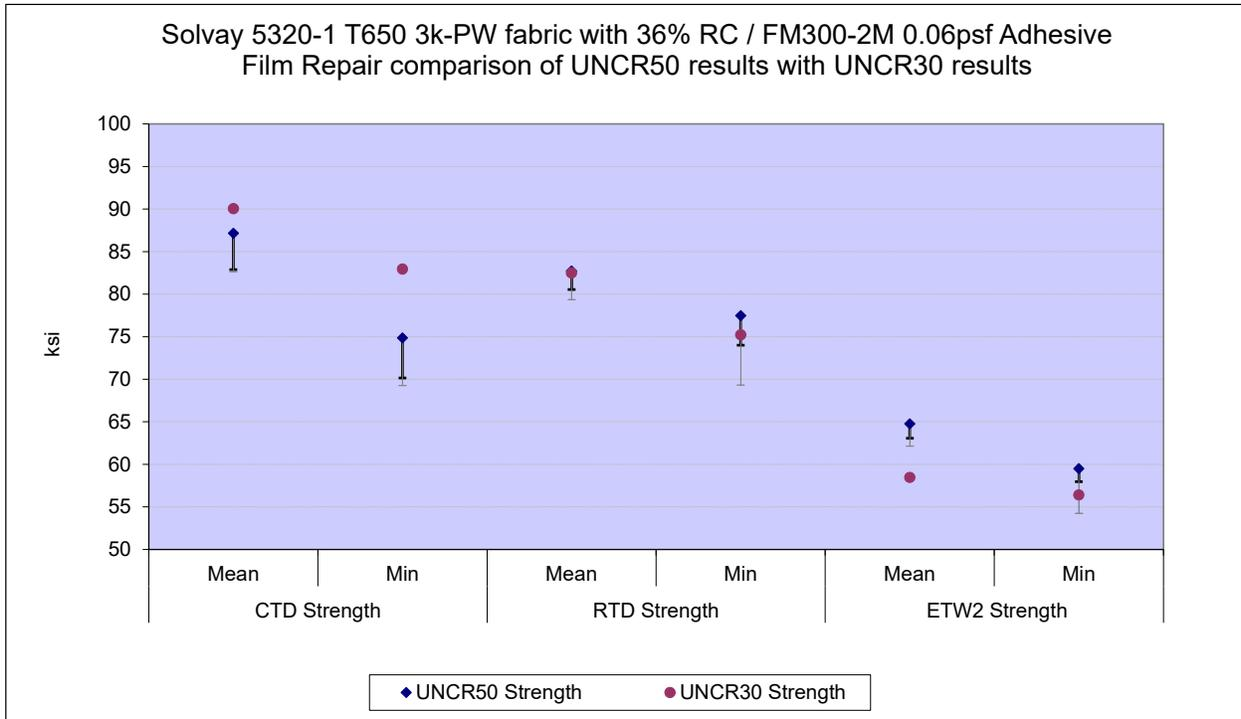
Figure 4-6: UNCR50 and UNCR30 Strength means, minimums and Equivalence Limits
