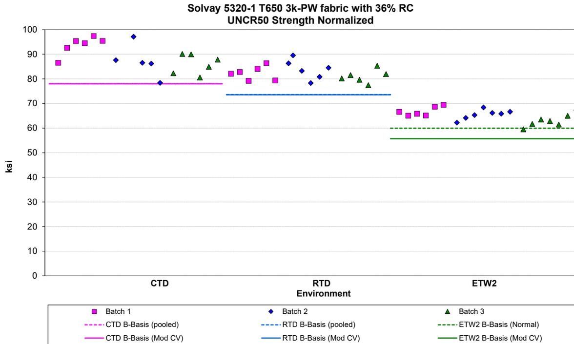
**Figure 4-2: Batch Plot for UNCR50 Strength Normalized**
