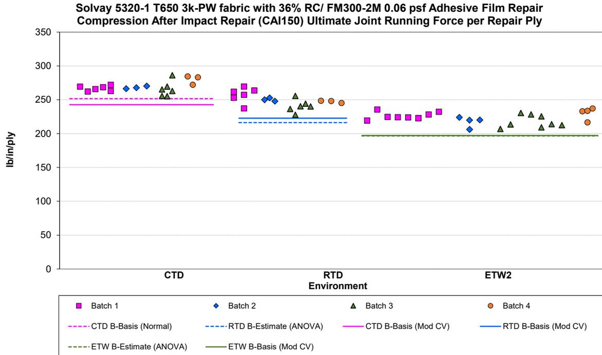
**Figure 4-14: Batch Plot for CAI150 Ultimate Joint Running Force per Repair Ply As-measured**
