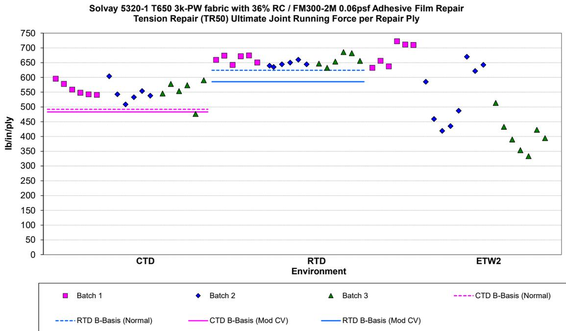
**Figure 4-9: Batch plot for TR50 Ultimate Joint Running Force per Repair Ply As-measured**
