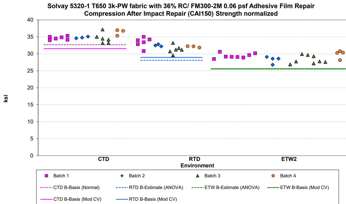
Figure 4-13: Batch Plot for CAI150 Strength normalized
