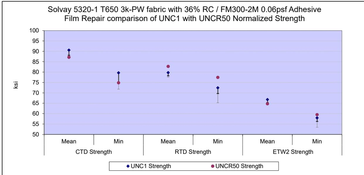
Figure 4-4: UNC1 and UNCR50 Strength means, minimums and Equivalence limits
