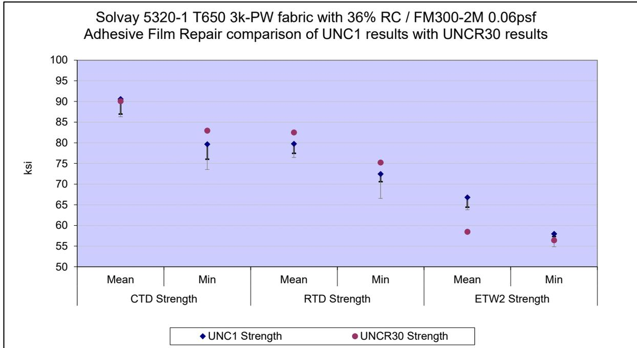
Figure 4-5: UNC1 and UNCR30 Strength means, minimums and Equivalence Limits
