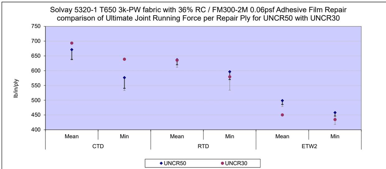
Figure 4-7: UNCR50 and UNCR30 Ultimate Joint Running Force per Repair Ply means, minimums and Equivalence Limits
