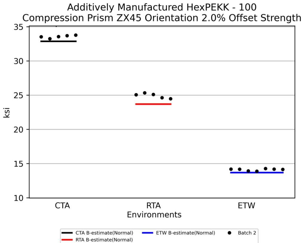
Figure 4-7: Batch Plot for Compression Prism ZX45 Orientation 2.0% Offset Strength
