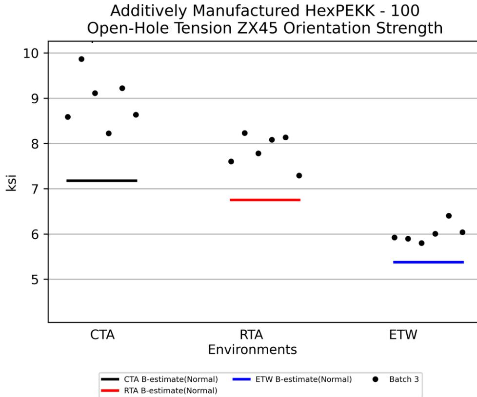
**Figure 4-52: Plot for OHT ZX45 Orientation Strength**
