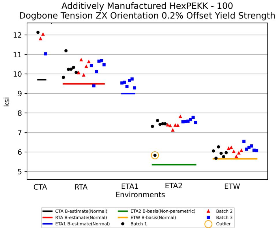
Figure 4-15: Batch plot for Dogbone Tension ZX Orientation 0.2% Offset Strength
