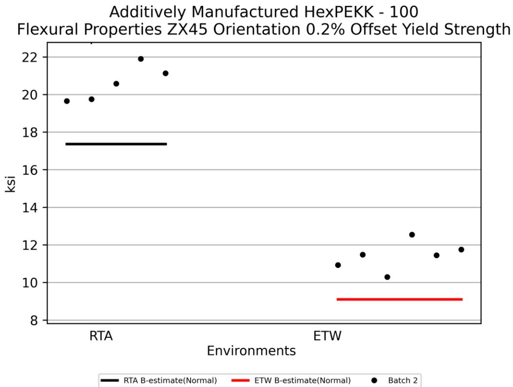
**Figure 4-36: Plot for Flex ZX45 Orientation 0.2% Offset Yield Strength**
