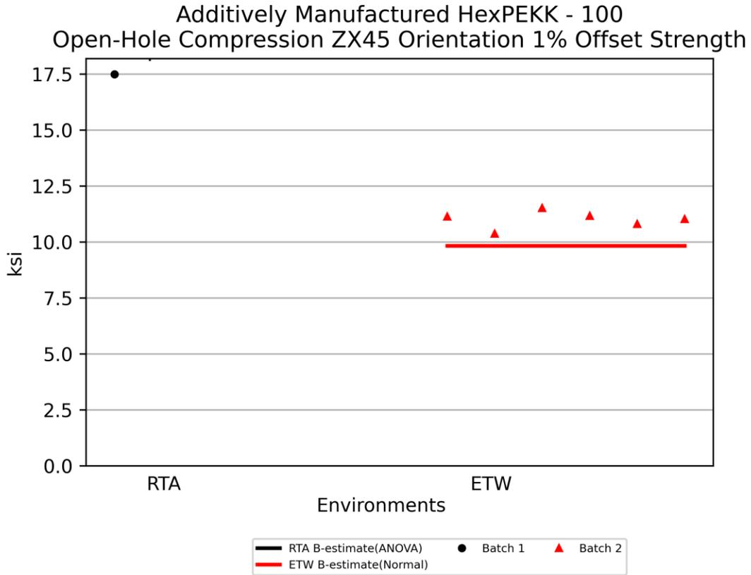
**Figure 4-47: Plot for OHC ZX45 Orientation 1% Offset Strength**
