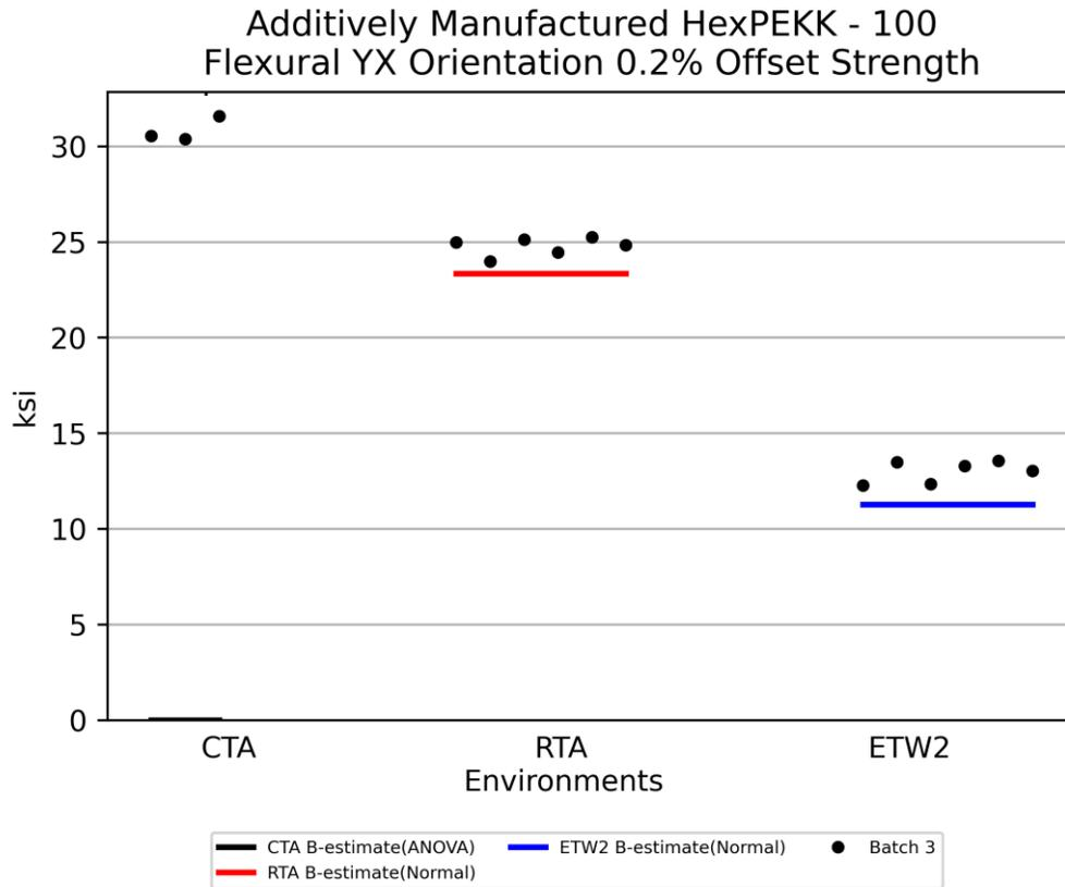
Figure 4-33: Plot for Flex YX Orientation 0.2% Offset Yield Strength
