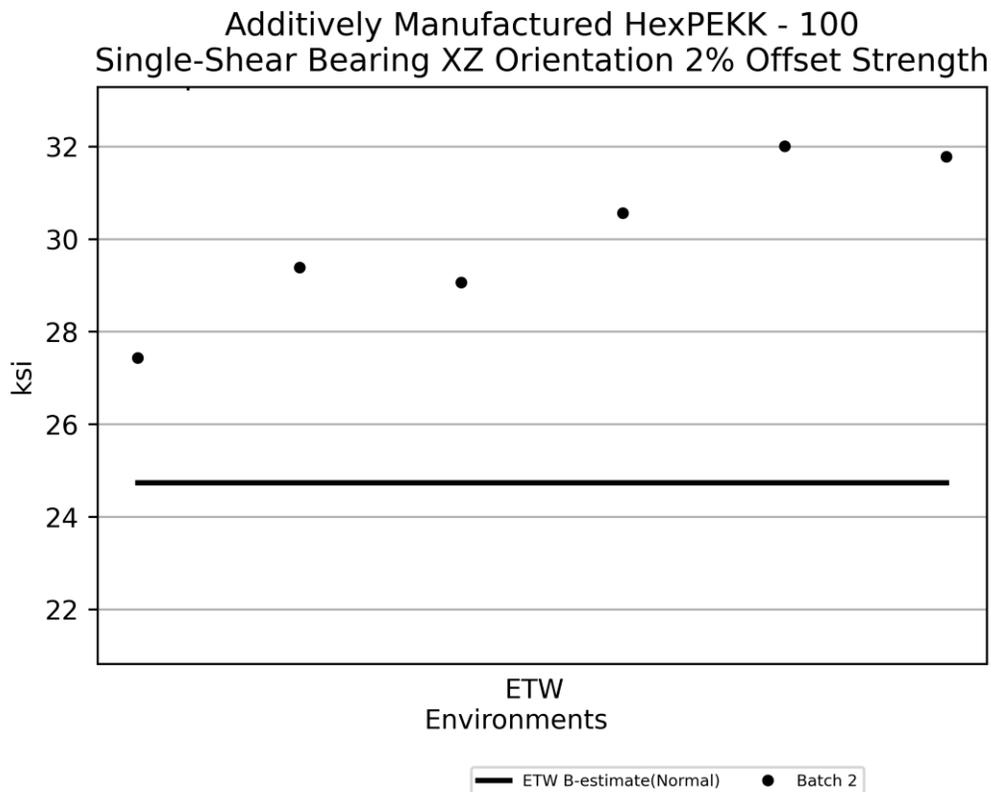
**Figure 4-58: Plot for SSB XZ Orientation 2% Offset Strength**
