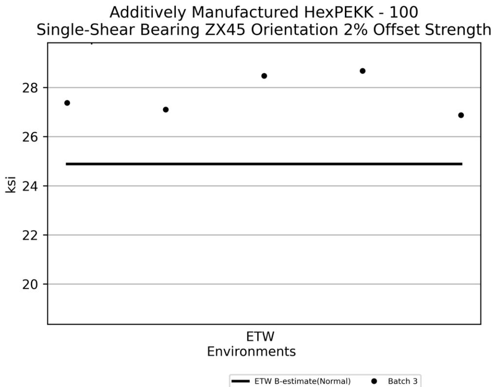
**Figure 4-64: Plot for SSB ZX45 Orientation 2% Offset Strength**
