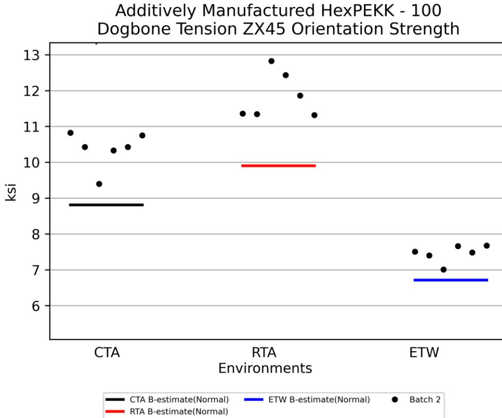
Figure 4-18: Batch plot for Dogbone Tension ZX45 Orientation Strength
