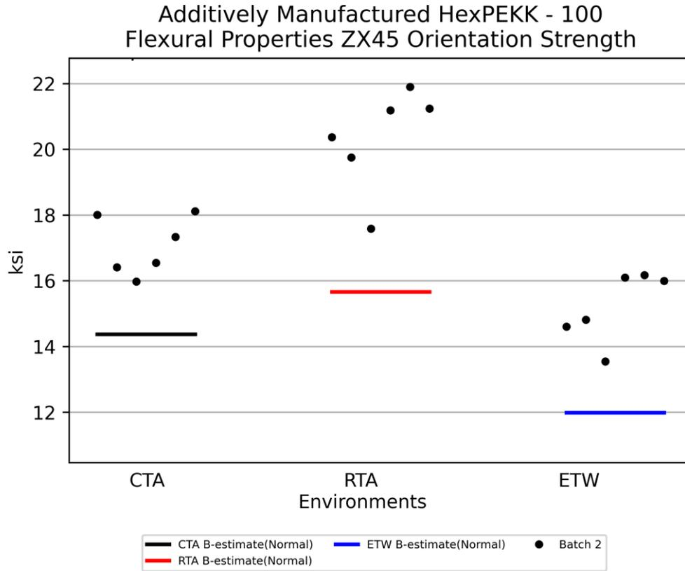
**Figure 4-37: Plot for Flex ZX45 Orientation Strength**
