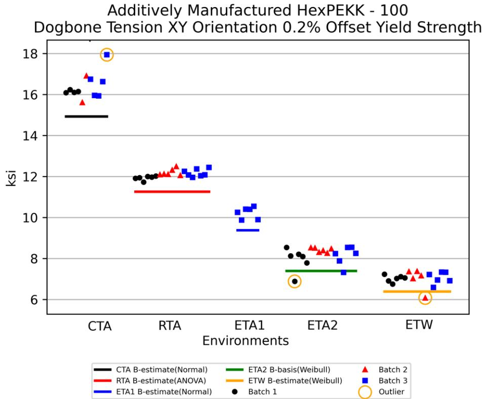
Figure 4-9: Batch plot for Dogbone Tension XY Orientation 0.2% Offset Yield Strength
