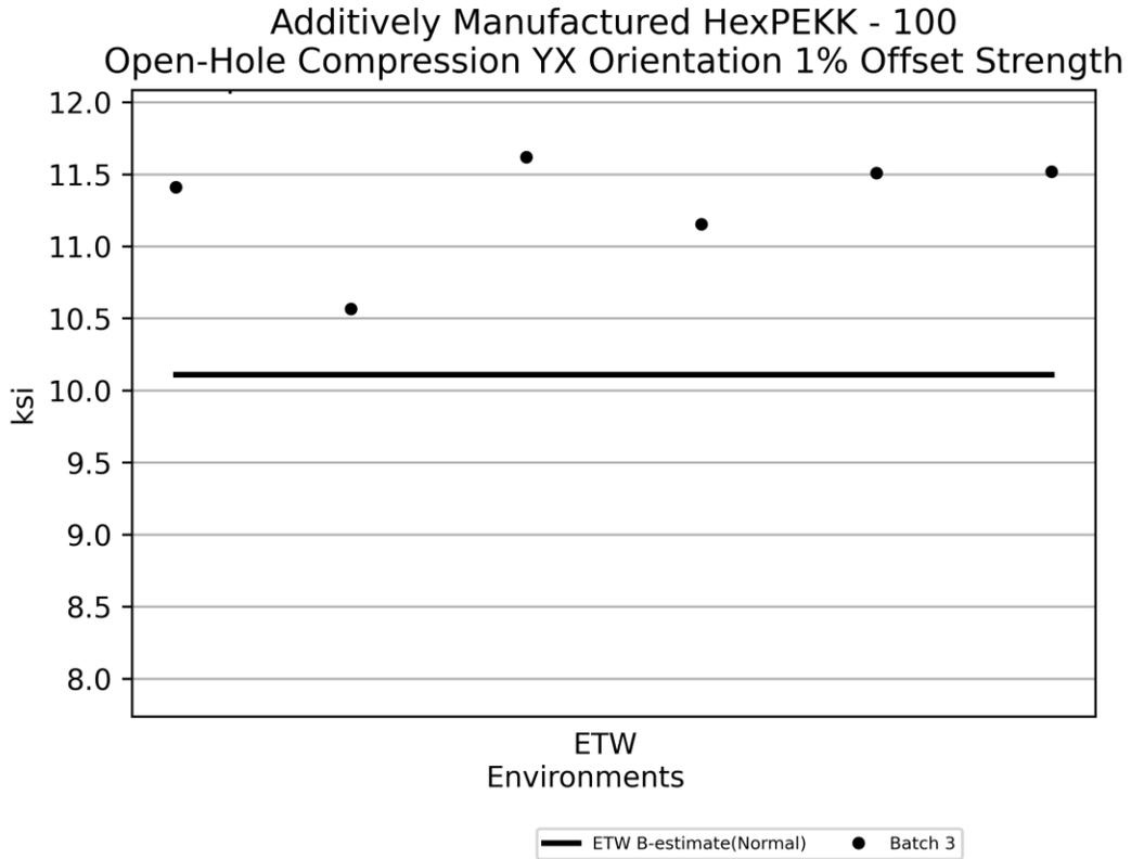
**Figure 4-43: Plot for OHC YX Orientation 1% Offset Strength**
