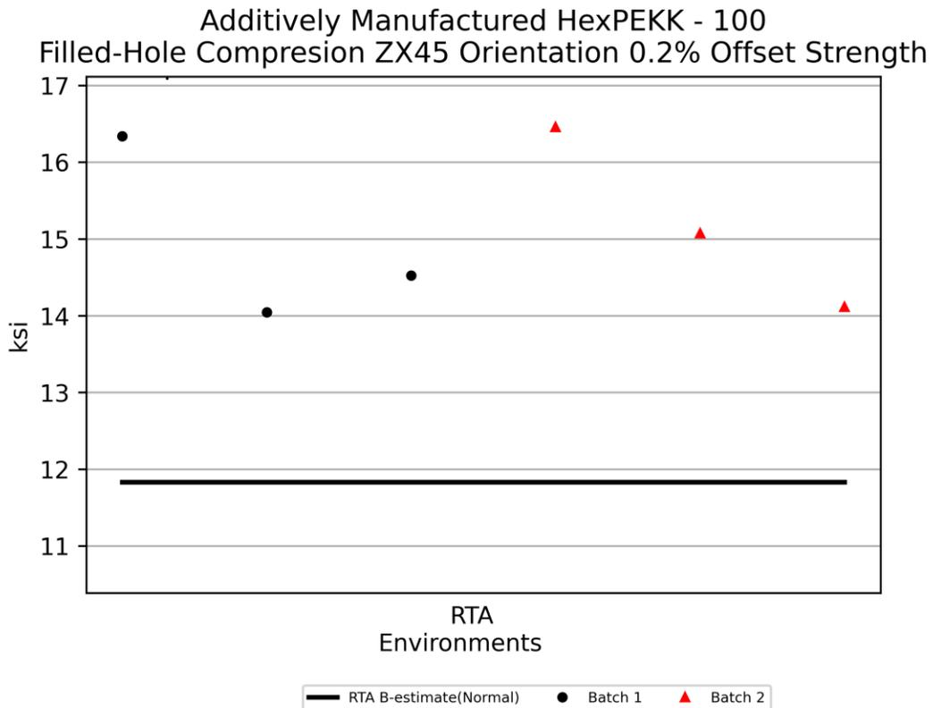
Figure 4-21: Batch plot for FHC ZX45 Orientation 0.2% Offset Strength
