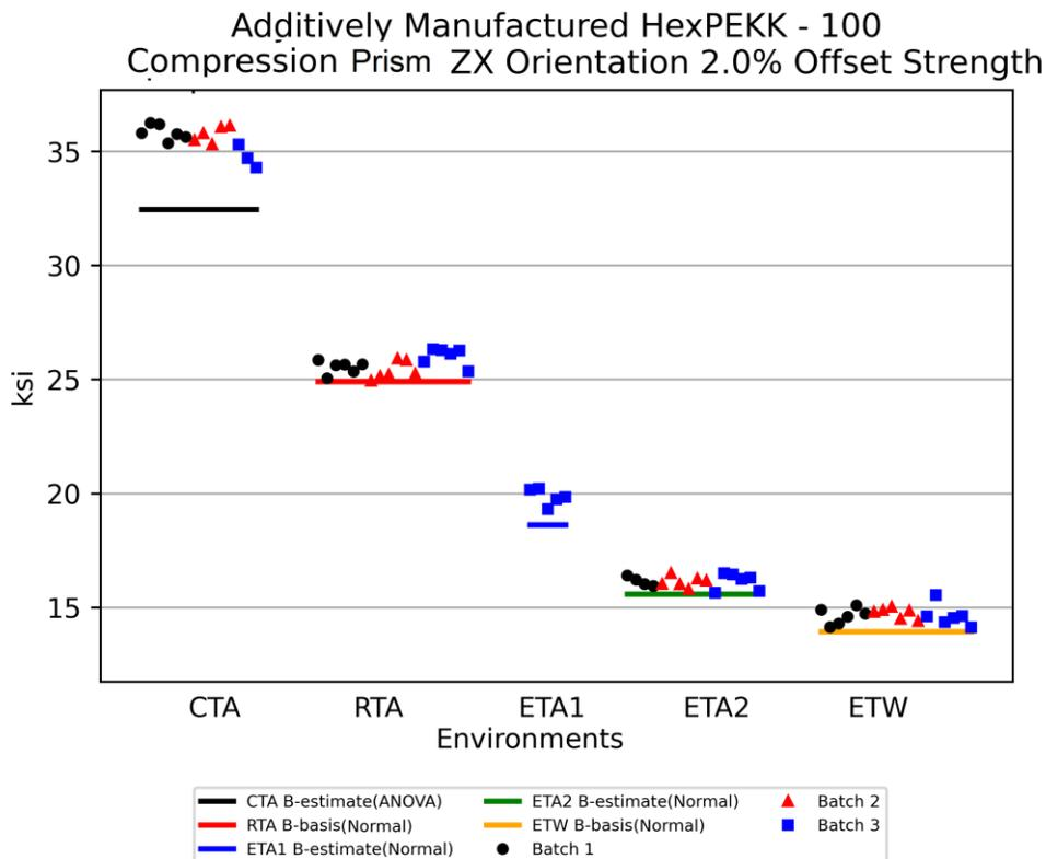
Figure 4-5: Batch Plot for Compression Prism ZX Orientation 2.0% Offset Strength
