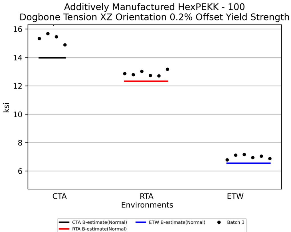
**Figure 4-11: Batch plot for Dogbone Tension XZ Orientation 0.2% Offset Yield Strength**
