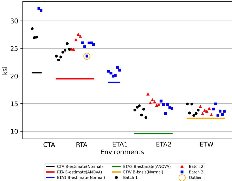
Figure 4-29: Plot for Flex XY Orientation 0.2% Offset Yield Strength
