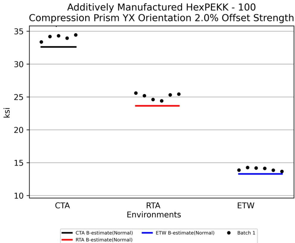
**Figure 4-3: Batch Plot for Compression Prism YX Orientation 2.0% Offset Strength**
