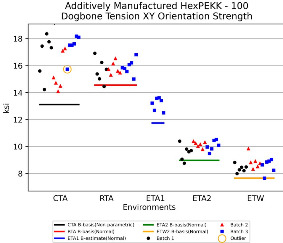
**Figure 4-10: Batch plot for Dogbone Tension XY Orientation Strength**
