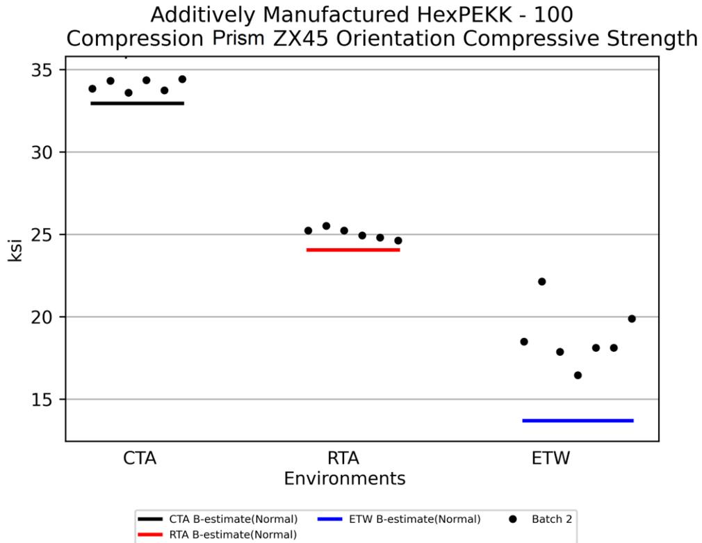
Figure 4-8: Batch Plot for Compression Prism ZX45 Orientation Compressive Strength
