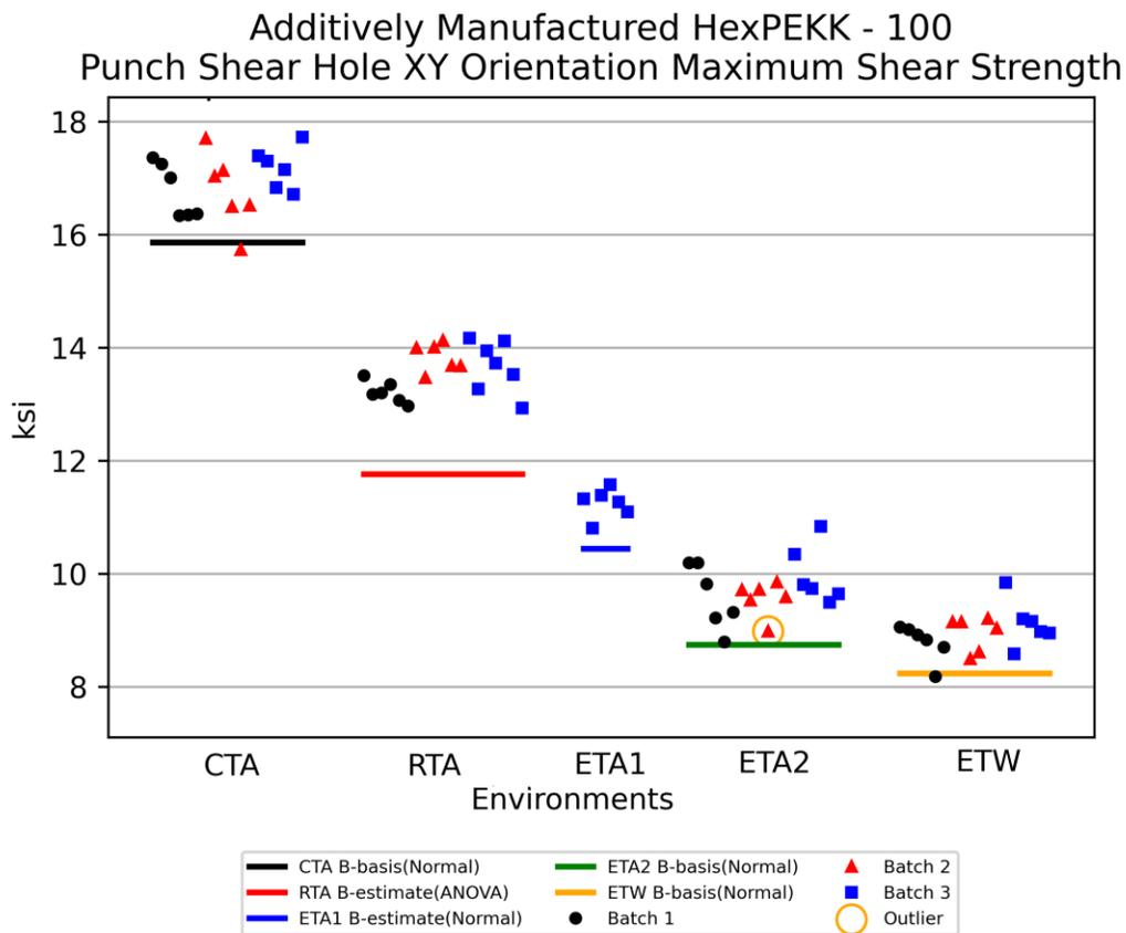
**Figure 4-53: Plot for PSH XY Orientation Maximum Shear Strength**
