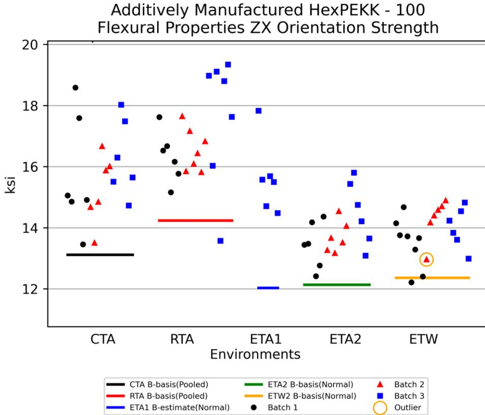
**Figure 4-36: Plot for Flex ZX Orientation Strength**
