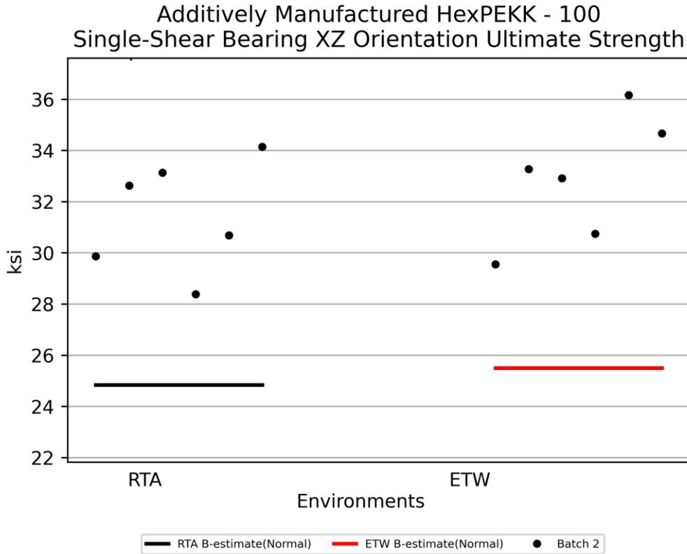
**Figure 4-59: Plot for SSB XZ Orientation Ultimate Strength**
