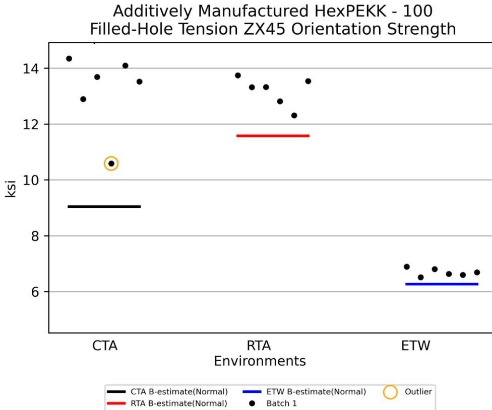
**Figure 4-28: Batch plot for FHT ZX45 Orientation Strength**
