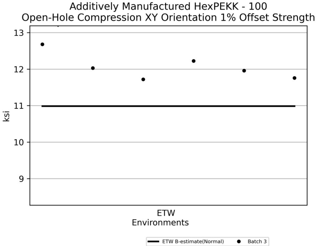
Figure 4-39: Plot for OHC XY Orientation 1% Offset Strength
