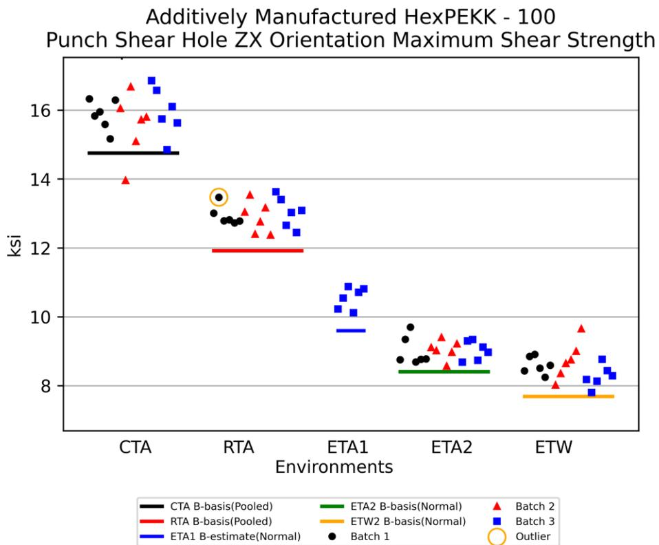
**Figure 4-54: Plot for PSH ZX Orientation Maximum Shear Strength**
