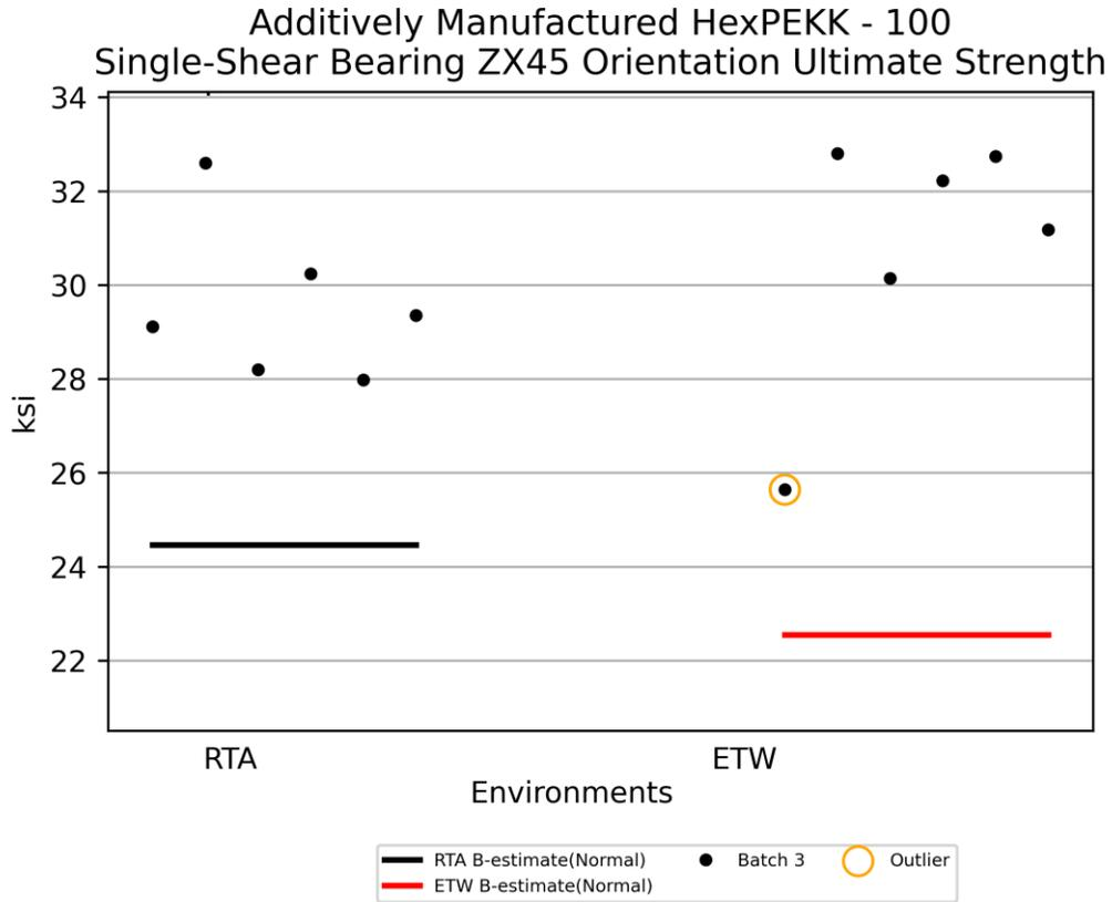
**Figure 4-65: Plot for SSB ZX45 Orientation Ultimate Strength**
