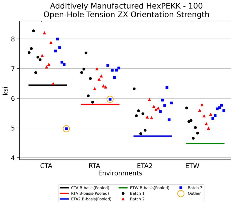
**Figure 4-51: Plot for OHT ZX Orientation Strength**
