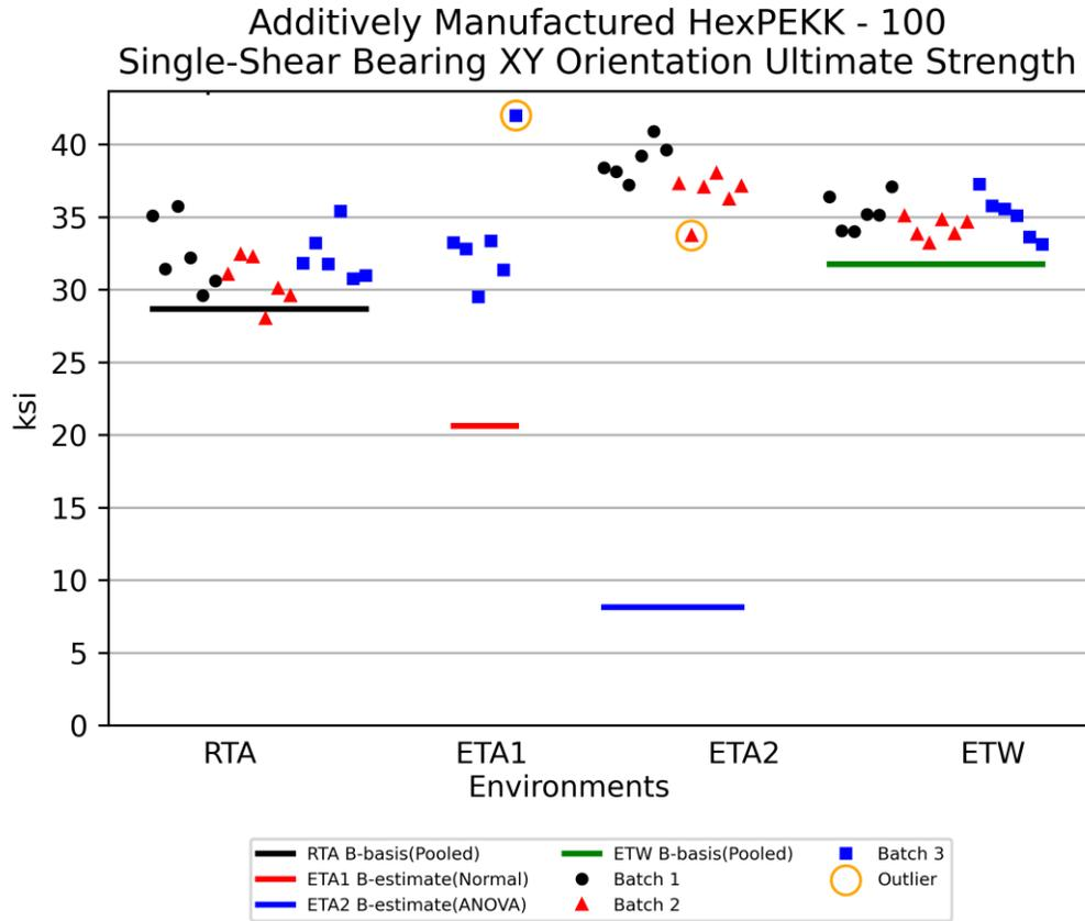
**Figure 4-57: Plot for SSB XY Orientation Ultimate Strength**
