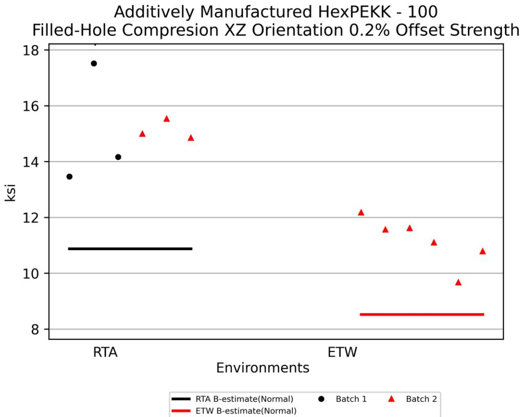
**Figure 4-19: Batch plot for FHC XZ Orientation 0.2% Offset Strength**
