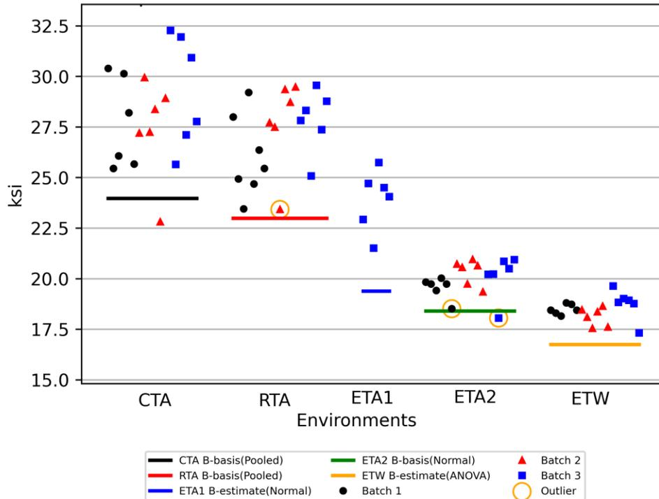
**Figure 4-30: Plot for Flex XY Orientation Strength**
