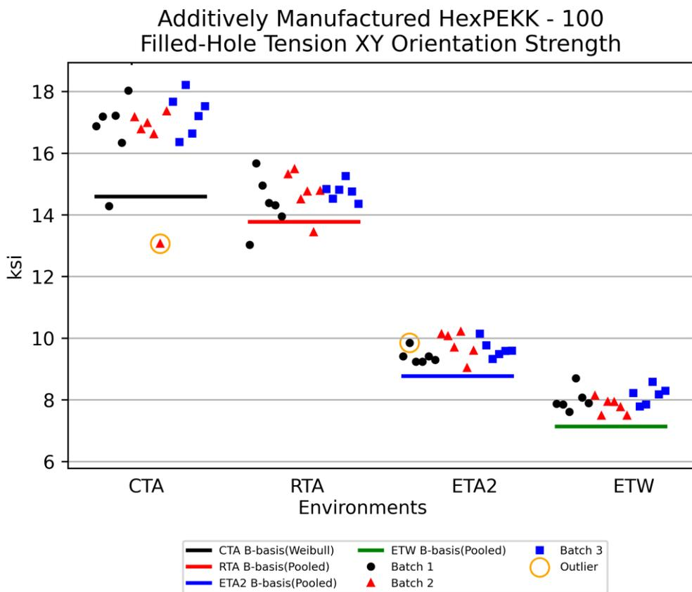
Figure 4-24: Batch plot for FHT XY Orientation Strength
