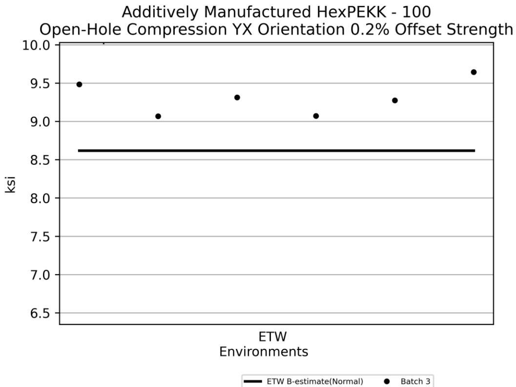
Figure 4-42: Plot for OHC YX Orientation 0.2% Offset Yield Strength
