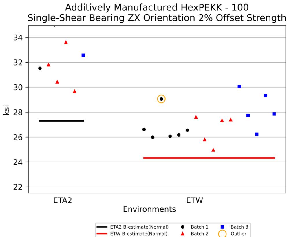
Figure 4-62: Plot for SSB ZX Orientation 2% Offset Strength
