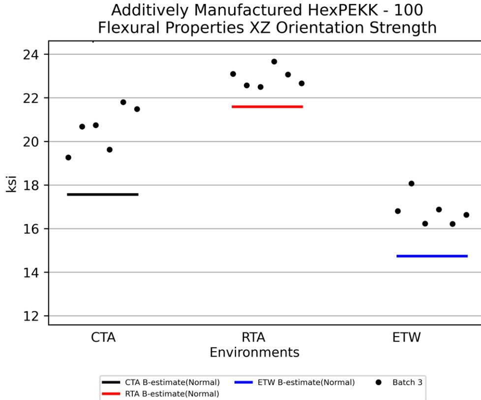
**Figure 4-32: Plot for Flex XZ Orientation Strength**
