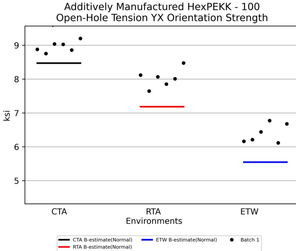
**Figure 4-50: Plot for OHT YX Orientation Strength**
