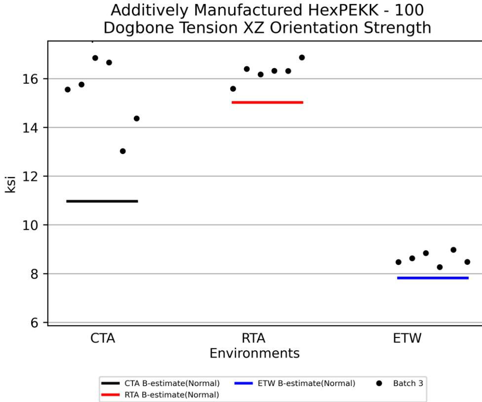
Figure 4-12: Batch plot for Dogbone Tension XZ Orientation Strength
