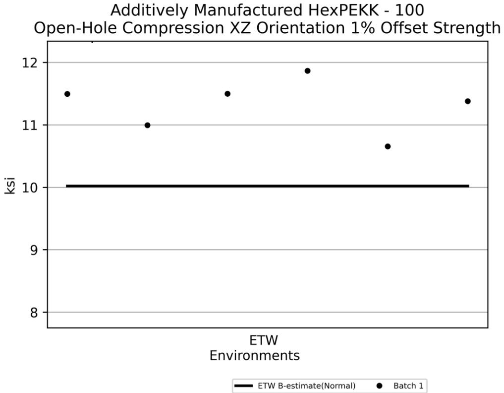
Figure 4-41: Plot for OHC XZ Orientation 1% Offset Strength
