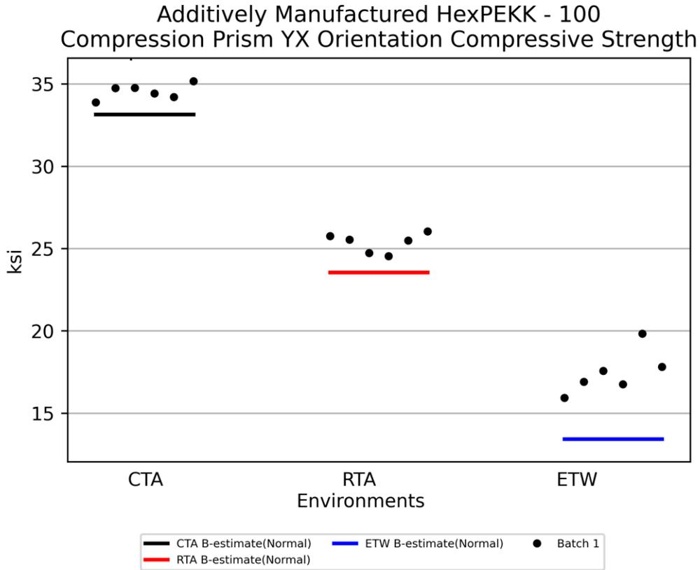
**Figure 4-4: Batch Plot for Compression Prism YX Orientation Compressive Strength**
