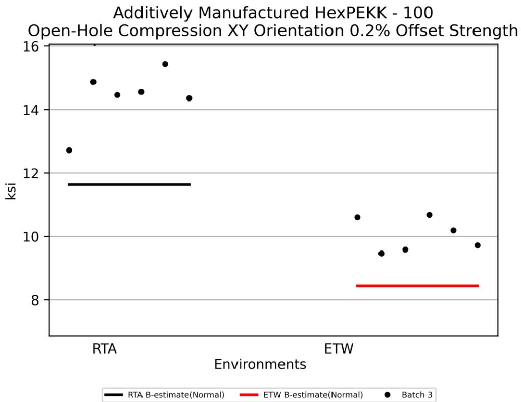
**Figure 4-38: Plot for OHC XY Orientation 0.2% Offset Yield Strength**
