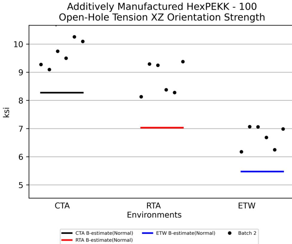
Figure 4-49: Plot for OHT XZ Orientation Strength
