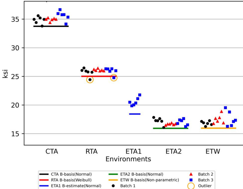
Figure 4-2: Batch plot for Compression Prism XY Orientation Compressive Strength
