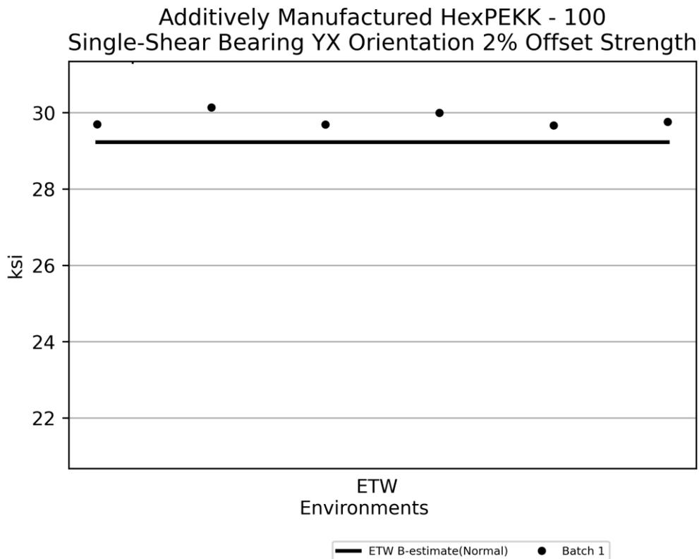
Figure 4-60: Plot for SSB YX Orientation 2% Offset Strength
