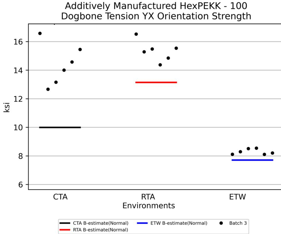
**Figure 4-14: Batch plot for Dogbone Tension YX Orientation Strength**
