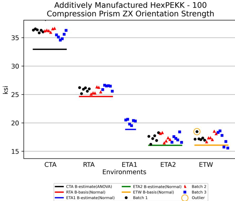
Figure 4-6: Batch Plot for Compression Prism ZX Orientation Compressive Strength
