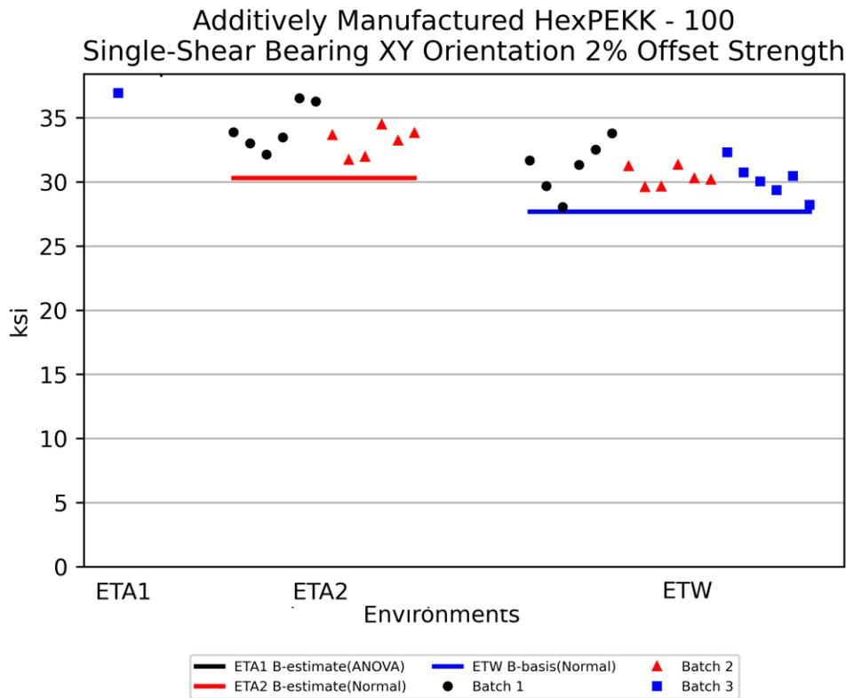
**Figure 4-56: Plot for SSB XY Orientation 2% Offset Strength**
