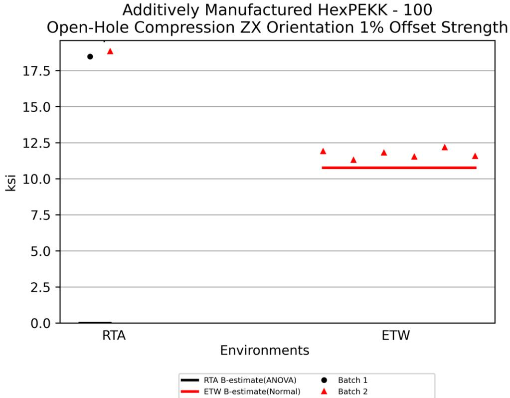
**Figure 4-45: Plot for OHC ZX Orientation 1% Offset Strength**
