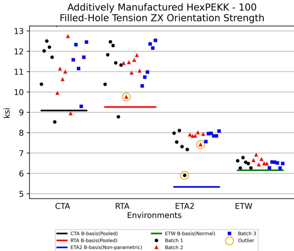
Figure 4-27: Batch plot for FHT ZX Orientation Strength
