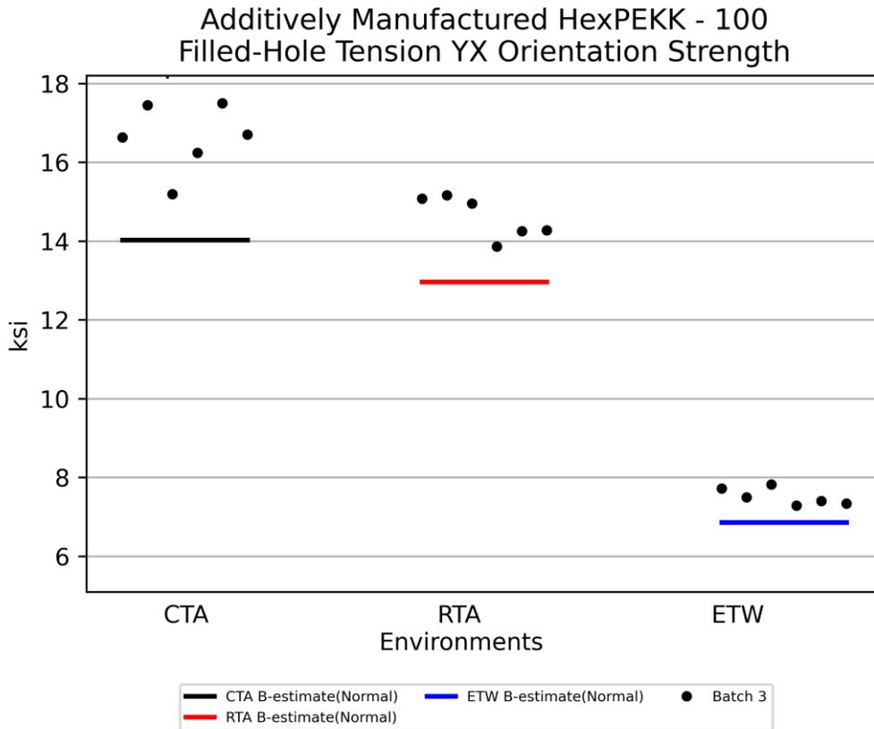
Figure 4-26: Batch plot for FHT YX Orientation Strength
