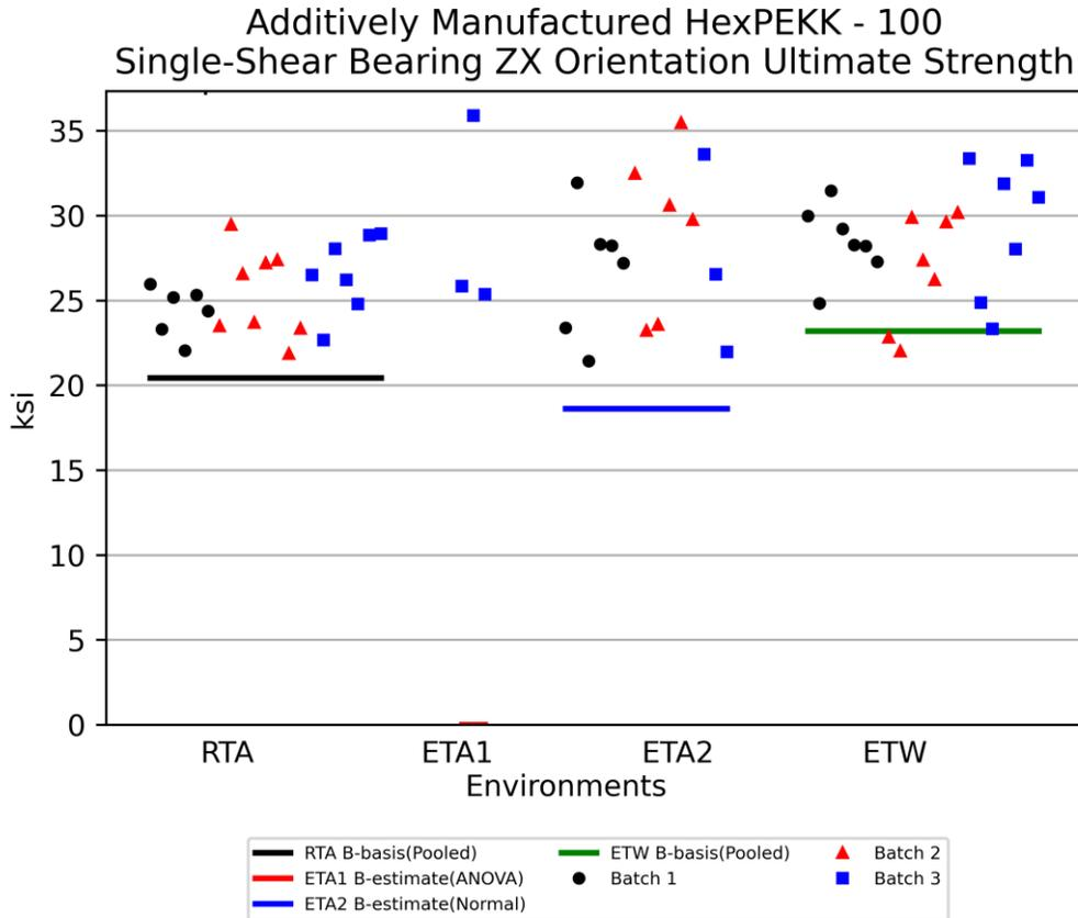
**Figure 4-63: Plot for SSB ZX Orientation Ultimate Strength**
