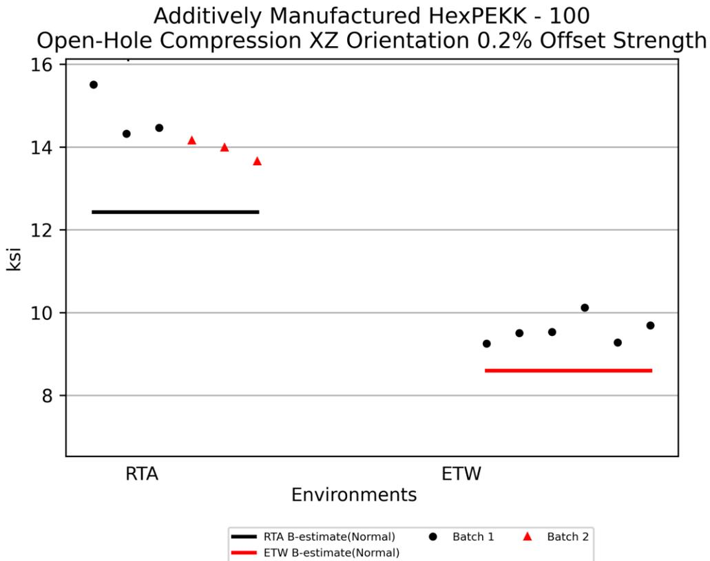
**Figure 4-40: Plot for OHC XZ Orientation 0.2% Offset Yield Strength**
