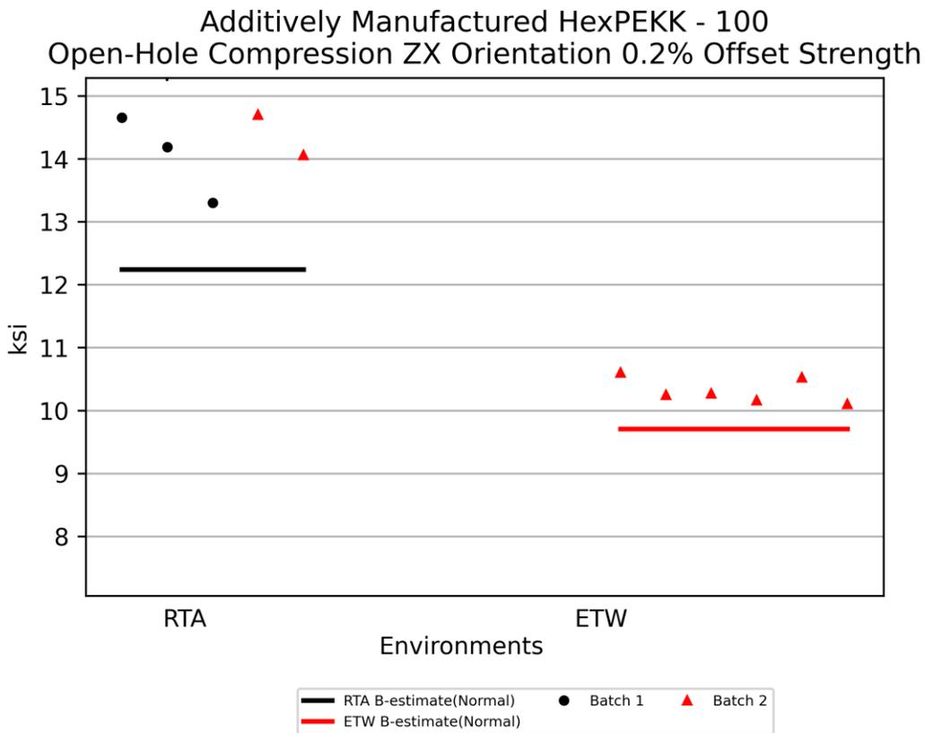
**Figure 4-44: Plot for OHC ZX Orientation 0.2% Offset Yield Strength**
