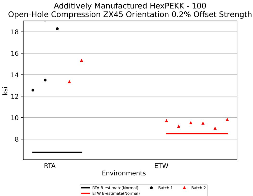
**Figure 4-46: Plot for OHC ZX45 Orientation 0.2% Offset Yield Strength**
