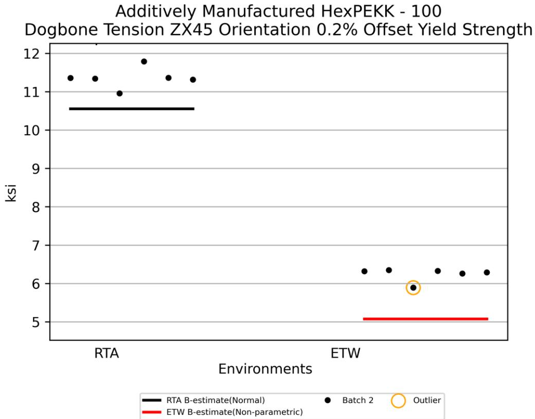
**Figure 4-17: Batch plot for Dogbone Tension ZX45 Orientation 0.2% Offset Strength**
