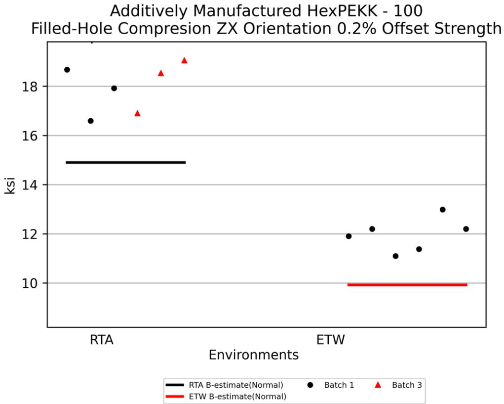
Figure 4-20: Batch plot for FHC ZX Orientation 0.2% Offset Strength
