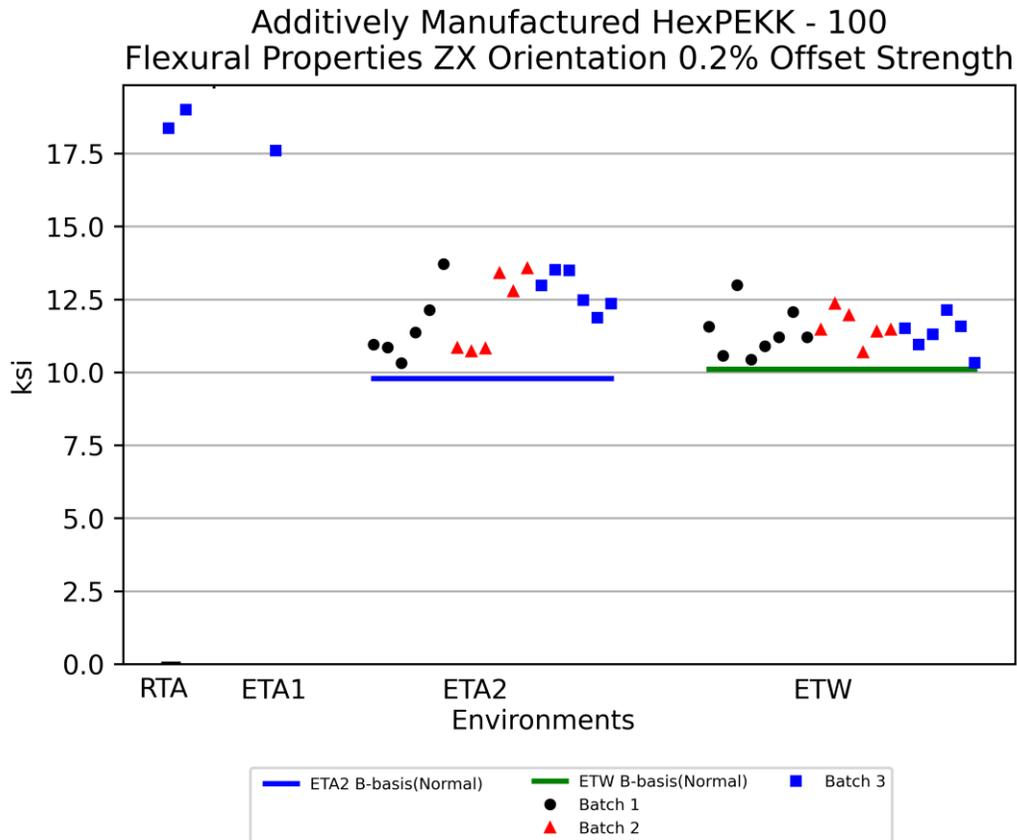
Figure 4-35: Plot for Flex ZX Orientation 0.2% Offset Yield Strength
