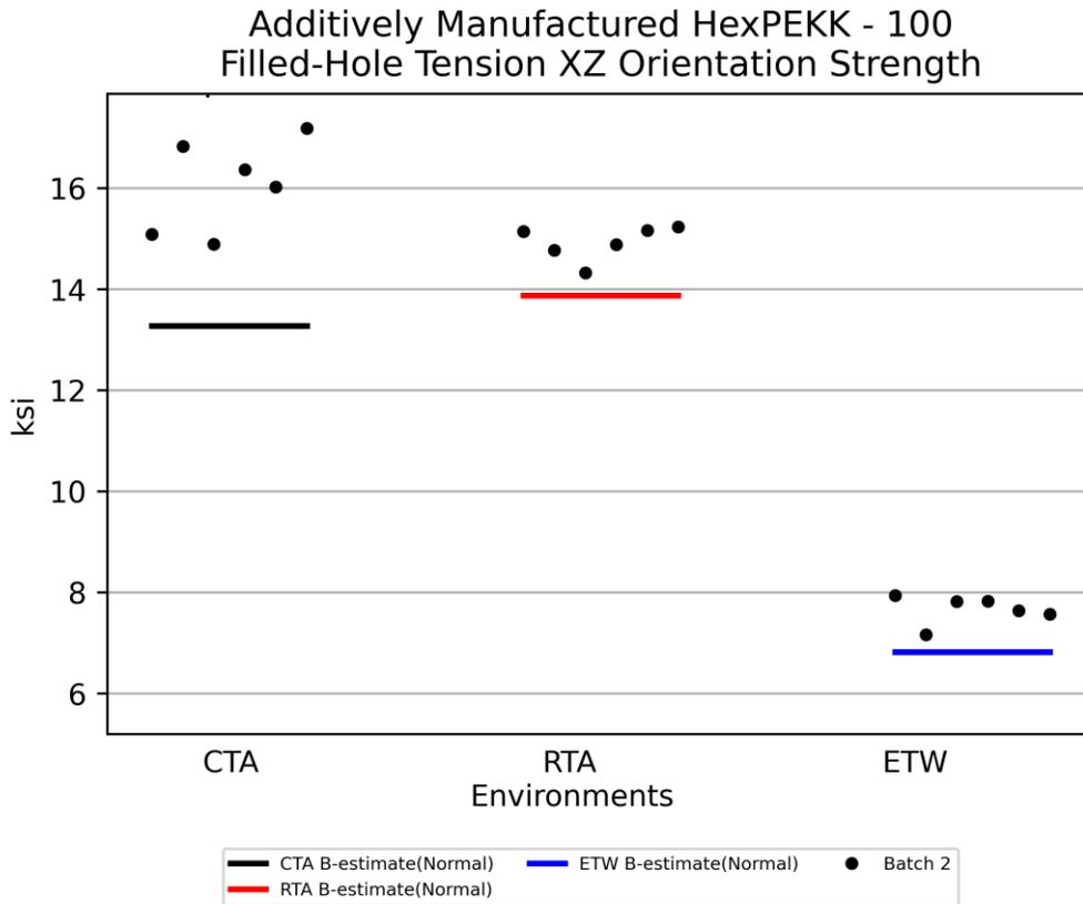
Figure 4-25: Batch plot for FHT XZ Orientation Strength
