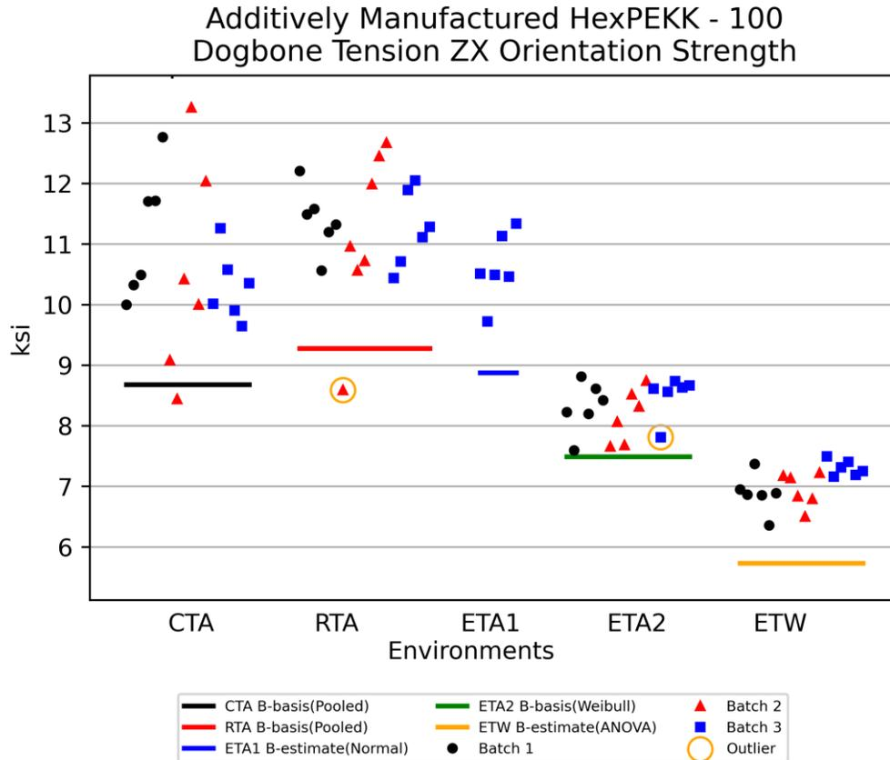
Figure 4-16: Batch plot for Dogbone Tension ZX Orientation Strength
