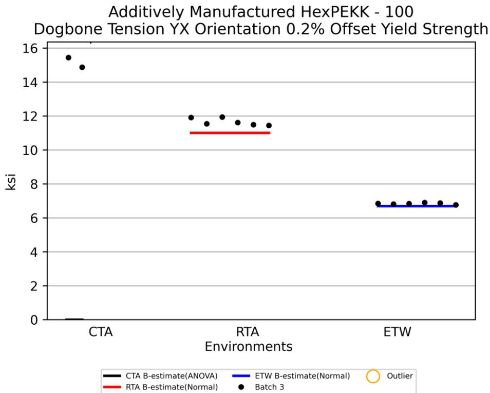
Figure 4-13: Batch plot for Dogbone Tension YX Orientation 0.2% Offset Yield Strength
