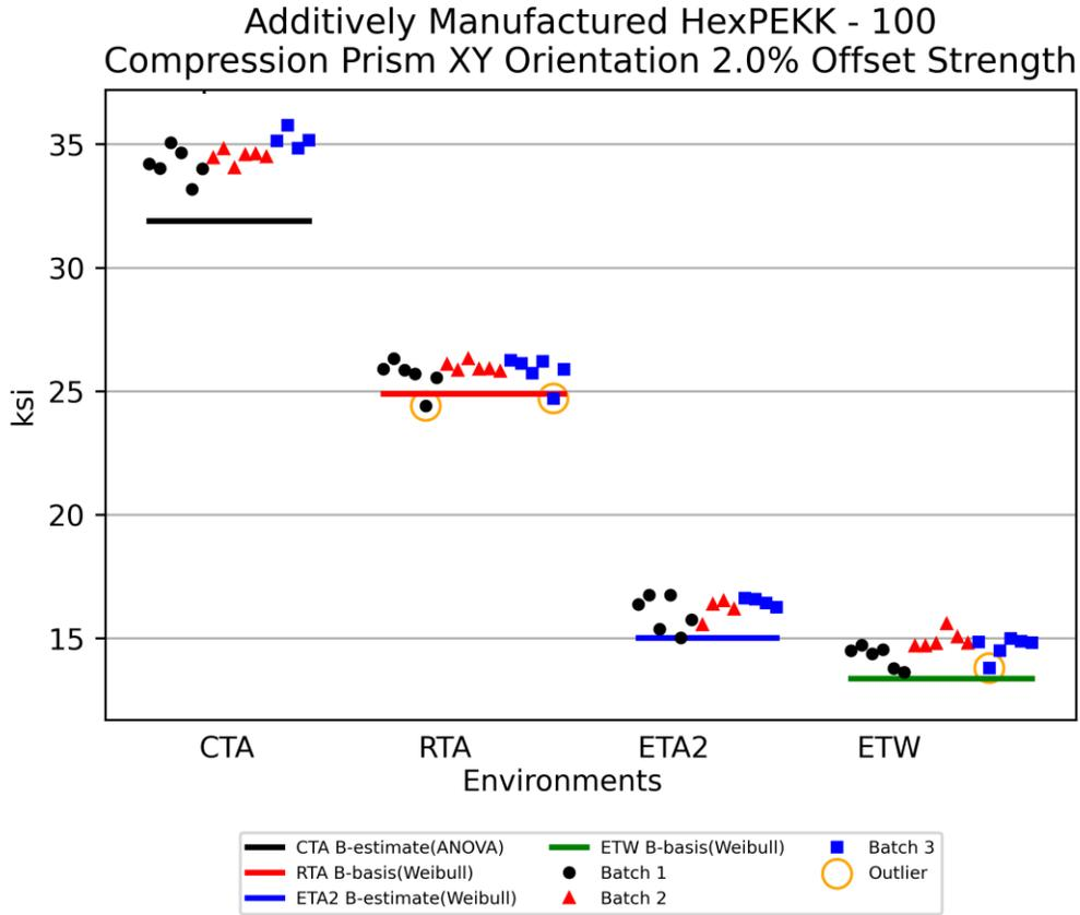
Figure 4-1: Batch plot for Compression Prism XY Orientation 2% Offset Strength
