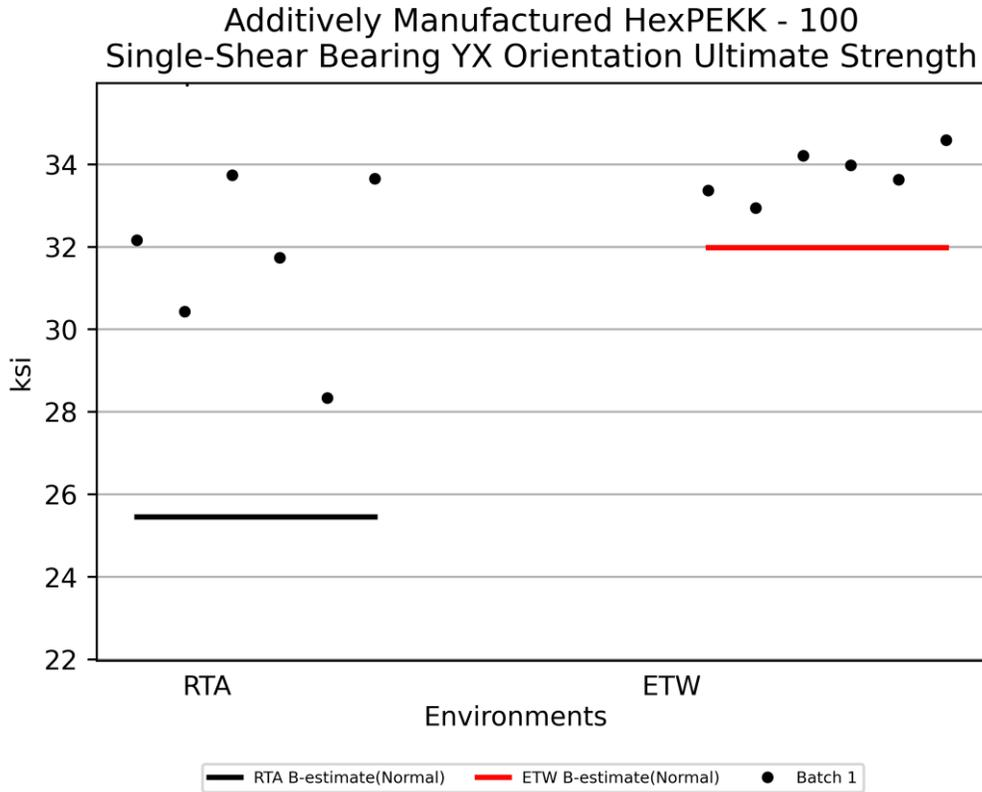
**Figure 4-61: Plot for SSB YX Orientation Ultimate Strength**
