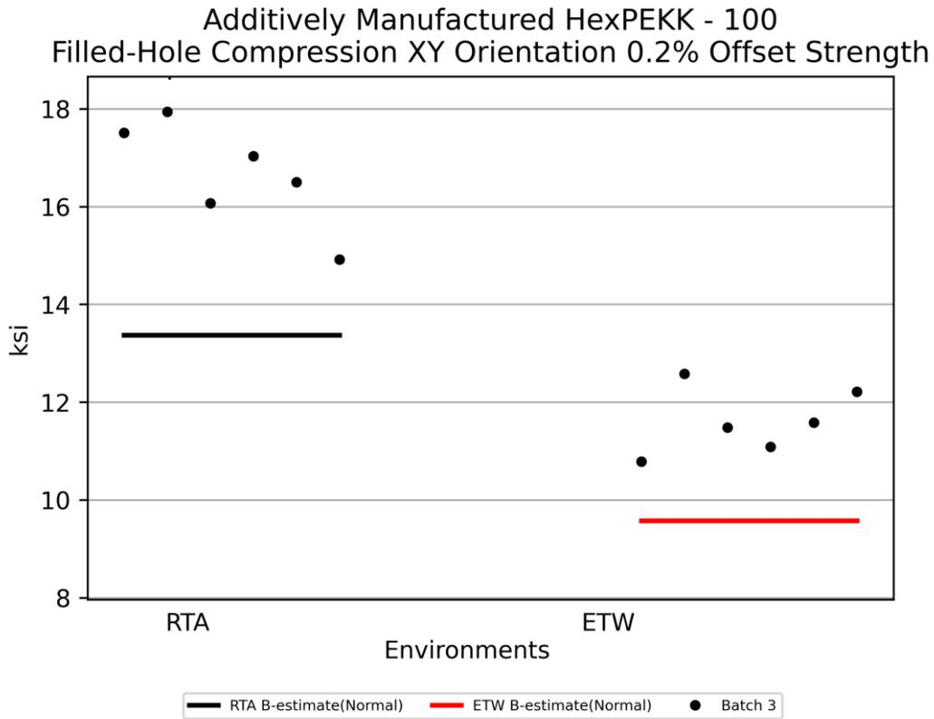
Figure 4-22: Batch plot for FHC XY Orientation 0.2% Offset Strength
