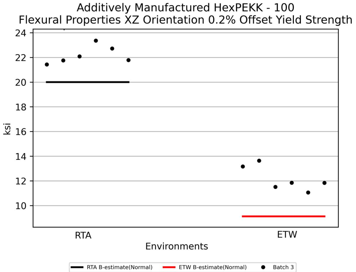
**Figure 4-31: Plot for Flex XZ Orientation 0.2% Offset Yield Strength**
