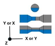
If more than one laser is used to build a specimen it may be counted for each laser independently and also as a combined laser stitched specimen. (e.g. a specimen produced using laser 2 and laser 4 can be used as a laser 2 specimen, laser 4 specimen, and a laser 2+4 stitched specimen).
