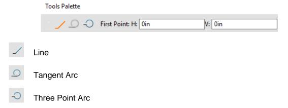
You will now perform a sketch with the Profile icon by using the Three Point Arc suboption. It allows you to define an arc without having to exit the Profile command.
