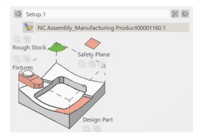
**Hide the stock part.** You can use the Hide/Show Stock icon. With the stock hidden, you can select the design part much easier. If you did not want to hide the stock, you could have also expanded the specification tree until you can access the part body of the design part.
