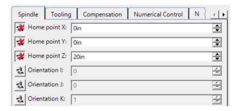
**Select** *OK***.** Always be sure the machine parameters are set properly, otherwise you will get inaccurate output in the APT generator, and thus you will get incorrect output in the final machine code.
