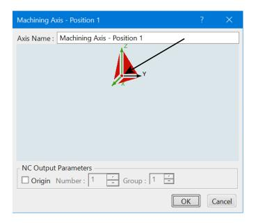
The center red dot will allow you to move the entire axis system from one location to another. The *Machining Axis System* window will disappear while CATIA waits for you to select a point or vertex to be the new center of the axis system.
