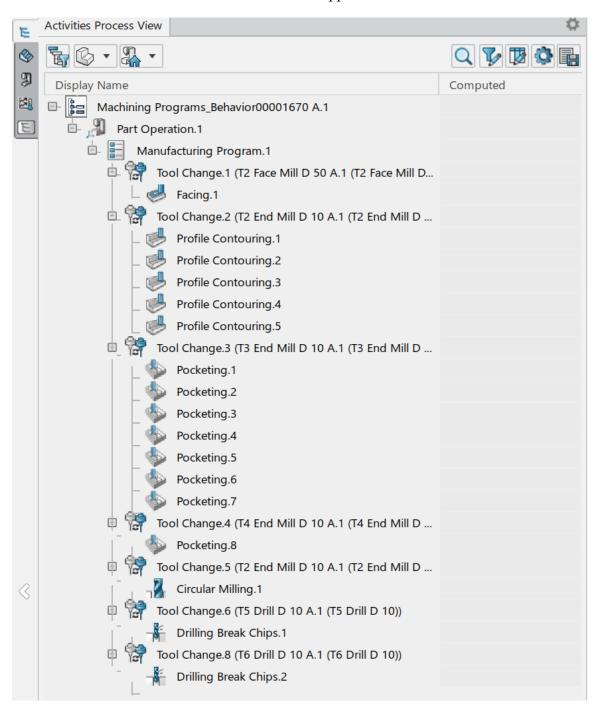
Machining operations can have two states. One state is to have the tool paths computed. In this state, the tool paths are available for the machining operation, and can be replayed instantly. When the tool paths are computed the green computed symbol will show up in the *Computed* column.
