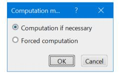
Computation if necessary This will compute the tool paths if the status of the tool path
