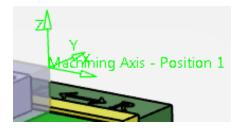
Notice the axis system in the machining axis window turns green. This denotes that a new axis location has been defined.
