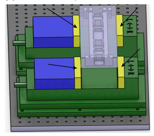
**Double select in the workspace when done.** You do not need to select on any part, just double select in space. You can define as many parts as fixture parts as you want. This will have four fixtures defined.
