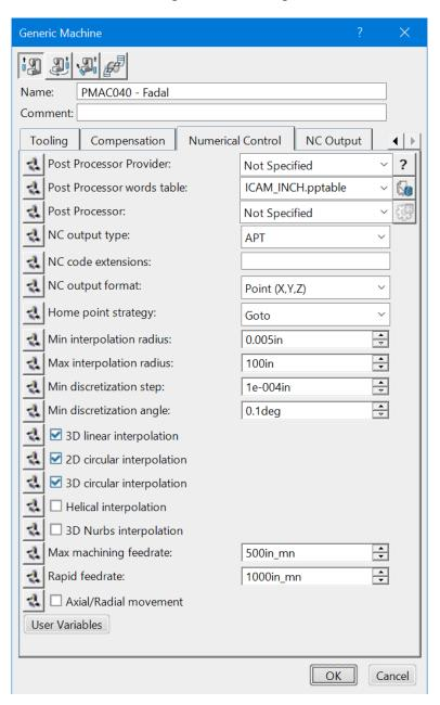
**Select** *OK* **when done.** This will have the machine set up. A part operation will appear in the tree.
