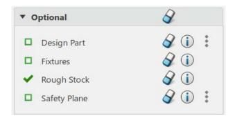
Hide the stock part. You can use the Hide/Show Stock icon. With the stock hidden, you can select the design part much easier. If you did not want to hide the stock, you could have also expanded the specification tree until you can access the part body of the design part.
