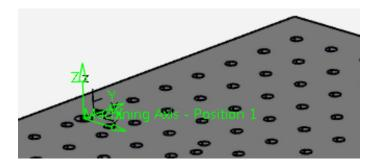
**Select** *OK* **to the machining axis window.** For now this will serve as the machining axis. Many times machine seeds will have an axis location defined that can serve as the machining axis.
