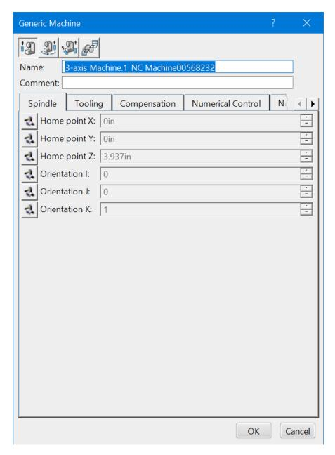
The first set of icons across the top allow you to define the specific type of machine you are going to be using.
