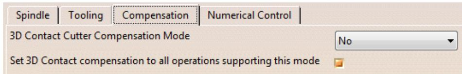
*3D Contact Cutter...* Defines the cutter compensation mode for cutting in 3D space
