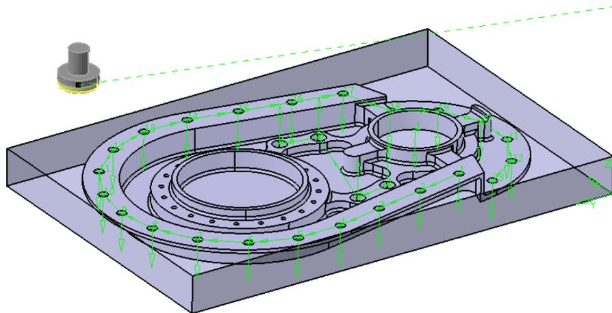
The only tool path displayed is the movement of the tool from the tool change point to the start of the tool paths. The transition motions are always shown in a dashed motion.
