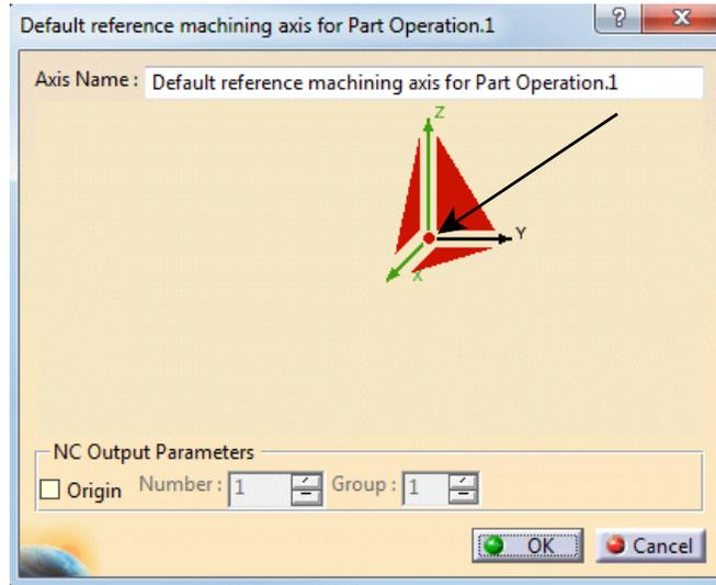
The center red dot will allow you to move the entire axis system from one location to another. The *Machining Axis System* window will disappear while CATIA waits for you to select a point or vertex to be the new center of the axis system.
