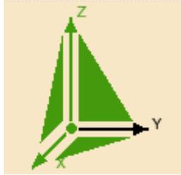
Now to adjust the axis directions. Assume in this case, you want the axis system pointing towards the part. This means that you want to reverse the X and Y axis directions such that they both point towards the stock part. Since you cannot change the Y axis, you will have to adjust the X axis direction.
