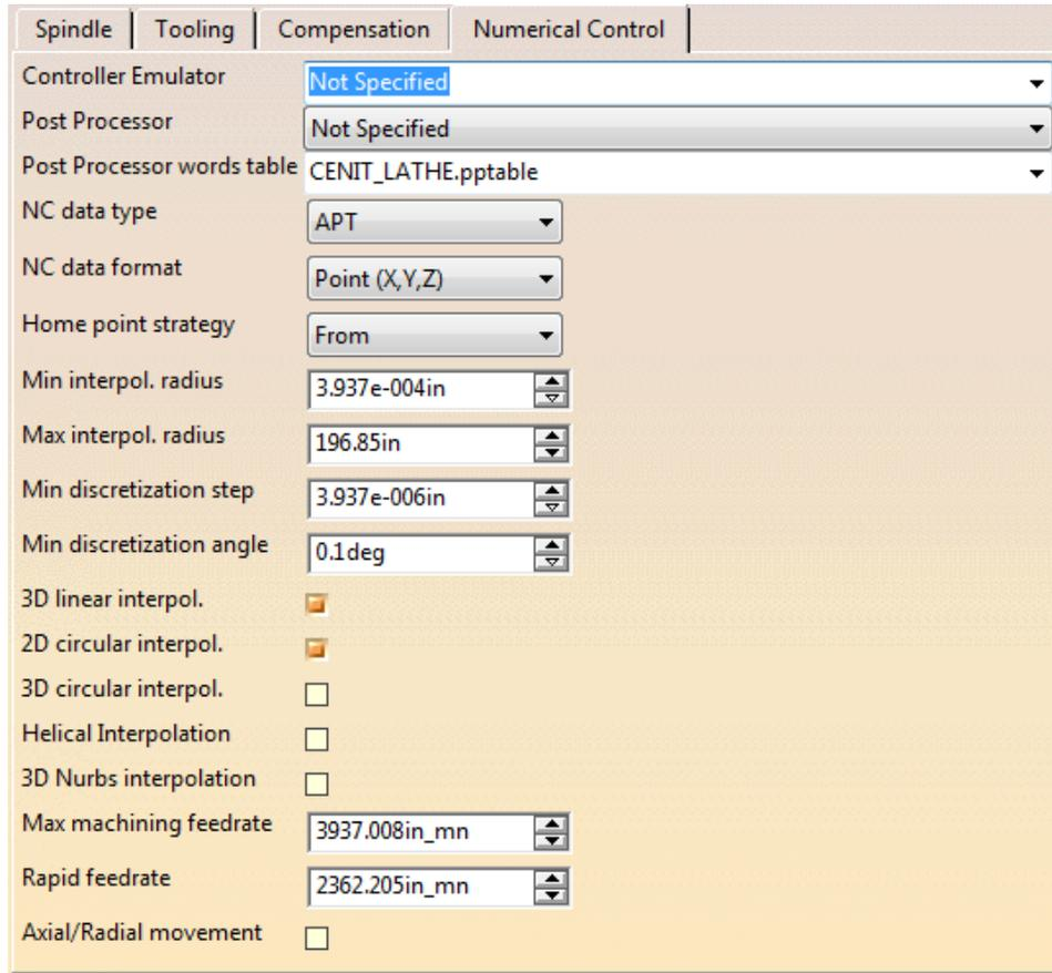
*Controller Emulator* Defines a controller emulator. The controller emulator allows machine simulation based on the post processed code.
