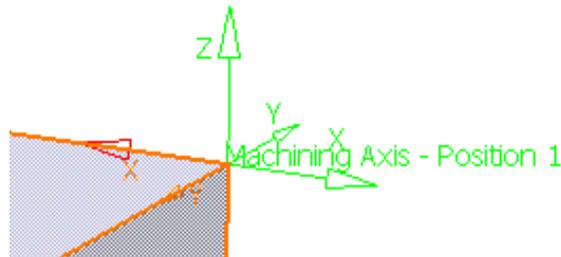
If you look very closely, you will notice faint red axis directions that indicate the new directions. Unfortunately, the green machining axis does not actually update until you complete the axis definition. You will find that many times you will need to complete the axis definition to insure the axis is correct. If it is not correct, then you will simply need to go back to the axis definition by selecting on the **Machining Axis** icon again.
