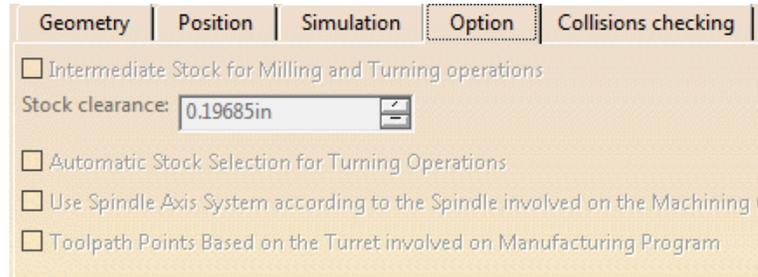
*Intermediate Stock...* Allows the intermediate stock to be automatically computed and taken into account for the tool path computation
