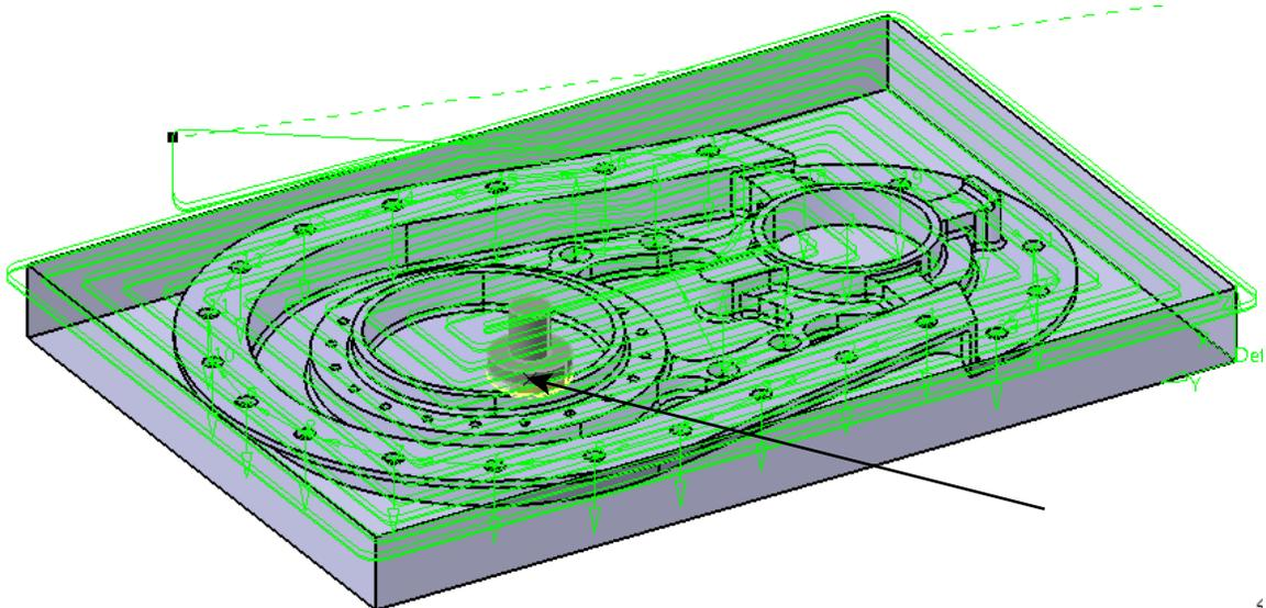
Having the tool follow the cursor can be beneficial to inspect tool position relative to the design part in a variety of different positions.
