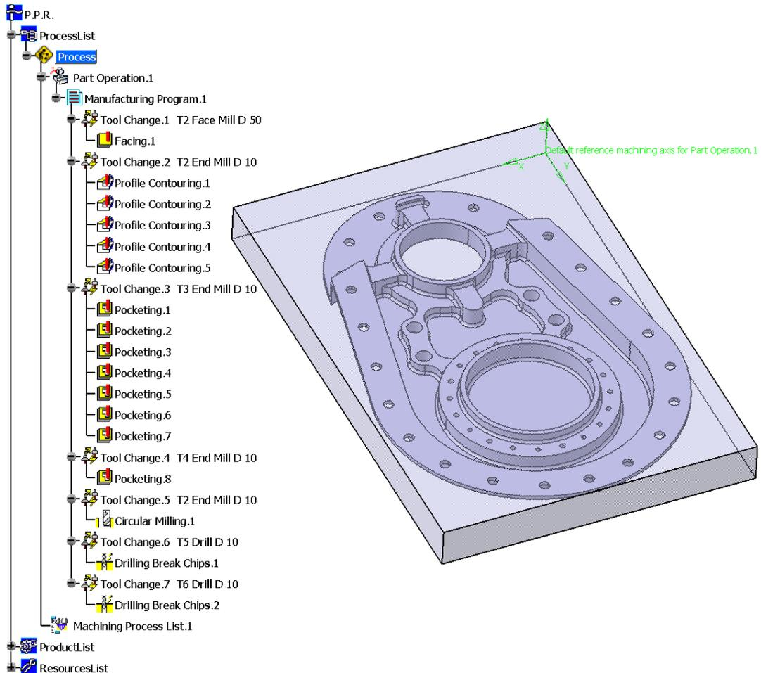
Machining operations can have two states. One state is to have the tool paths computed. In this state, the tool paths are available for the machining operation, and can be replayed instantly. When the tool paths are computed, a (*Computed*) text will appear next to the operation, and an additional branch will show up below the machining operation.
