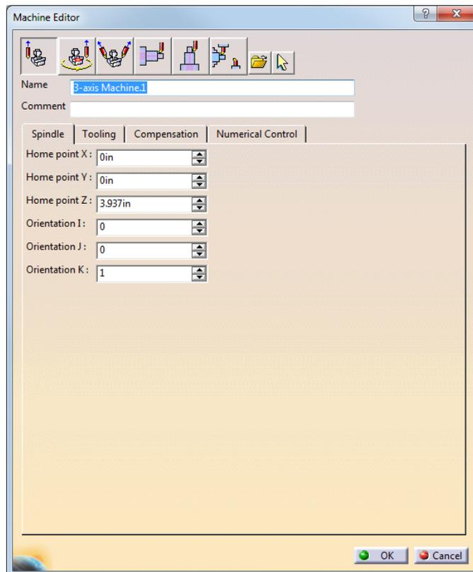
The first set of icons across the top allow you to define the specific type of machine you are going to be using.
