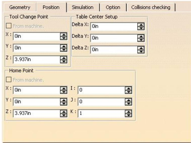
*Tool Change Point* Defines the X,Y,Z coordinates for the tool change point. This point should be away from the part, otherwise the tool will crash into the part to issue the tool change.
