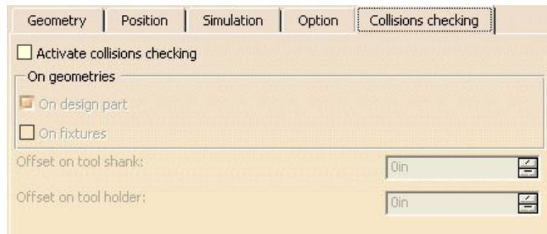
*Activate collisions...* Allows for quick feedback about collisions during the tool path replay
