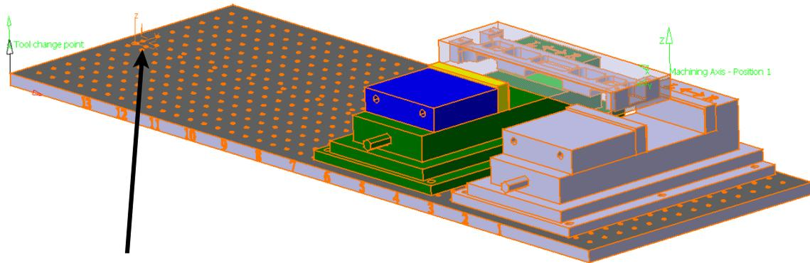
The machining axis will move and rotate to match the axis defined in the detail part.
