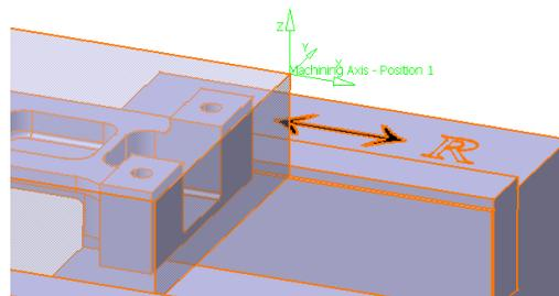
Notice the axis system in the machining axis window turns green. This denotes that a new axis location has been defined.
