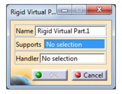
Select the inside of the four holes as shown to define the Supports for the virtual part. Make sure that you select the inner faces and not the edges.
