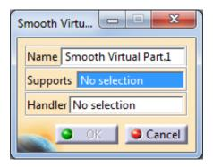
Select the inner faces of the two holes as shown to define the Supports for the virtual part.
