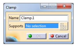
Select the rigid virtual part to define the Supports for the restraint. This will restrain the virtual part so that it cannot move at all.
