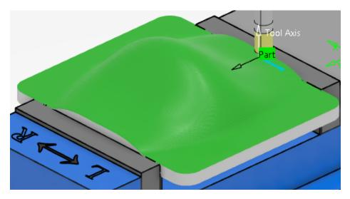
At this point, the surface quality is still rough, however, the machining parameters allow you to fine tune the tool paths to ensure a quality, smooth surface. Before adjusting machining parameters, take a moment to look at some of the additional geometry options.
