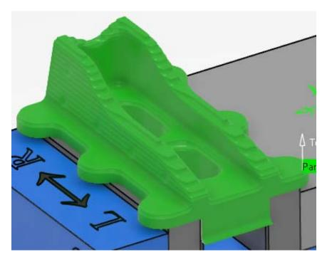
Select the *Imposed* definition and the planar face as shown. The imposed plane allows you to define flat planar areas that the tool will make a pass on. This is also helpful to define points that must be cut by the tool.
