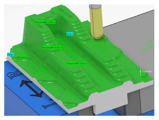
Generally, zone orders are used when you want to control the order of pocketing done in a large bulkhead. By default, in a large bulkhead with many pockets, the system will start at one end and work across the part, roughing in the most efficient manner. Although efficient, the part will gain considerable heat and may warp. By changing the order in which the pockets (zones) are machined, you can spread the heat build up around and avoid warping.
