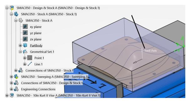
Select the Tool Axis definition. The Tool Axis window appears.
