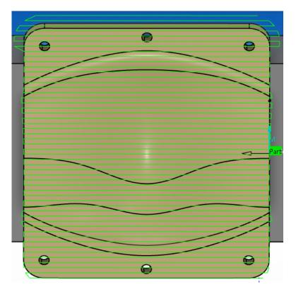
You should also notice that when you look directly down the line, you see straight, even, 0.25in paths all the way across the part. Again, this is due to the tool axis being changed such that the 0.25in constant tool paths are computed aligned to the tool axis.
