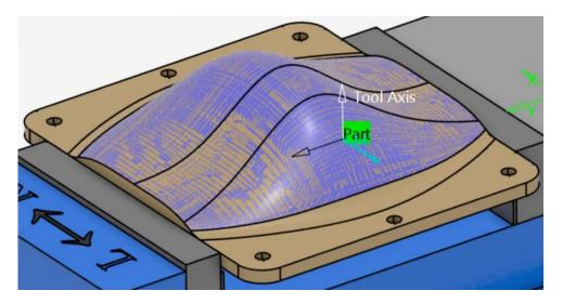
**Simulate the tool path.** Notice only the two surfaces get machined. Take a close look at the tool paths on the side. You should see that the tool paths do not conform to the contours of the faces selected.
