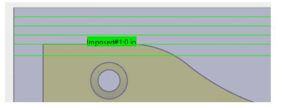
Even though you imposed the plane, the offset on part is always obeyed. This is why the tool does not cut across the top of the part.
