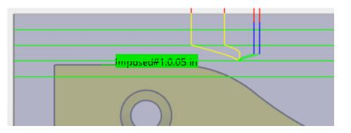
Even though you have added a 0.050in offset, the tool still does not cut at the imposed plane location. Until you make the imposed plane offset equal the Offset on part the tool will not cut at the imposed plane.
