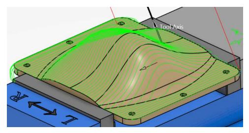
The tool paths along the flat surface are nearly the same as what you had before. Notice this time though, the tool paths extend down the side of the part and are more even against the side of the part.
