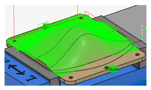
**Remove both the** *Start* and *End* options. This will go back to machining the entire surface.
