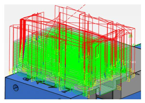
**Change offset value for the** *Part* **definition to be 0.125in.** This will tell the roughing operation to leave an 1/8th inch on the part surface. The surfaces will be finished with other operations.
