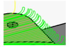
Set the *Between passes* macro to *High speed milling* with the following parameters. This is will define a 0.375in radius at the end of each pass, then move vertically 0.25in before circling around and returning to the part.
