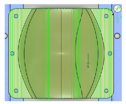
**Change the** *Stepover* **side to** *Left.* Notice the tool starts in the back left side, then steps right. You should also notice the blue machining direction axis change sides in the workspace. You can also flip the stepover side by selecting this axis.
