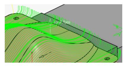
Notice that this takes care of all the "bad" locations that were left behind before. Through the combination of the between passes and between passes link macros, you can obtain full high speed milling motions at the end of the passes.
