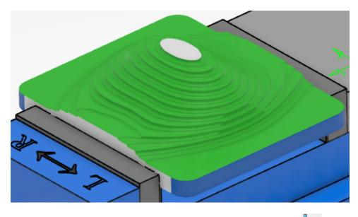
**Start a Sweeping operation after the profile contouring operation.** Whe Tool Axis window appears.
