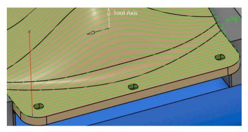
This can be impacted by modifying the tool axis. First, you will want to get a ball nose tool which will allow for better machining with a modified tool axis.
