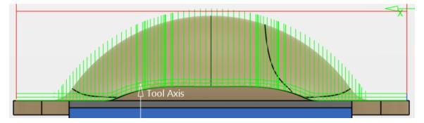
Since this is a purely vertical offset, it does not work very well to remove excessive material. You are better off to remove the excessive material with a sweep roughing operation prior to the sweeping operation, or to define multiple sweeping operations with part offsets.
