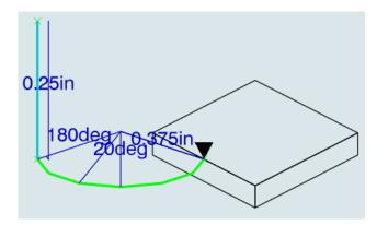
Simulate the tool paths. Now all of the paths move off the part before machining in the opposite direction.
