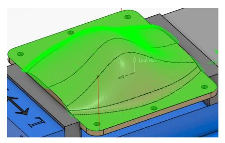
Change the *Tool path style* to *One-way next*. This will simply cause the tool to start on one side, then machine only in one direction.
