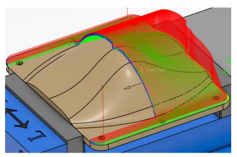
Not allowing the tool to plunge is good if you want to machine upwards along the part surface. By turning off the plunge, the tool will stop at the highest point, allowing you to go back and machine the opposite side without using limiting contours.
