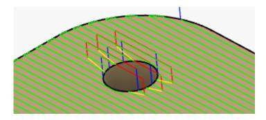
**Turn on the** *Direct* **option under the** *Zone* **tab.** Once you turn on direct, you have the ability to define the *Feedrate length*. If you remember from earlier, the *Feedrate length* defines the size of a gap the tool will cross in a direct motion.
