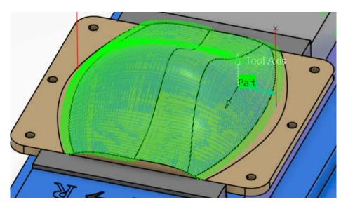
No matter the geometry of the part or faces that you want to machine, you will find that the tool paths are always straight and parallel.
