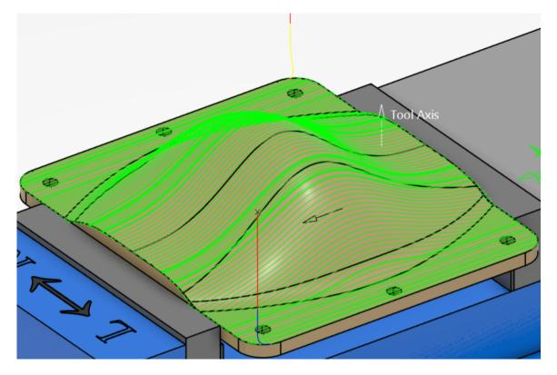
Set the *Between passes link* macro to *High speed milling* with a 0.25in *Transition Radius*. This will indicate that you wish to have a high speed milling motion between the passes with a 0.25in radius off the part. If the *Between passes* macro is not defined, there may be some situations where not all of the paths will have the radius.
