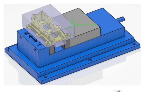
**Select the Roughing icon and select** *Manufacturing Program.1.* The *Tool Assembly Search* window appears. A tool assembly must be defined in order to create the operation.
