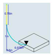
Change the *Retract* macro to a circular macro, with the *Angular sector* at 90deg, the *Angular orientation* at 90deg, the *Radius* at .5 and the axial distance at 1.0in. As you might have noticed, using the pre-defined macros allow for a quick definition of the macros. Many times it is advantageous to use the pre-defined macros instead of trying to custom build macros all the time.
