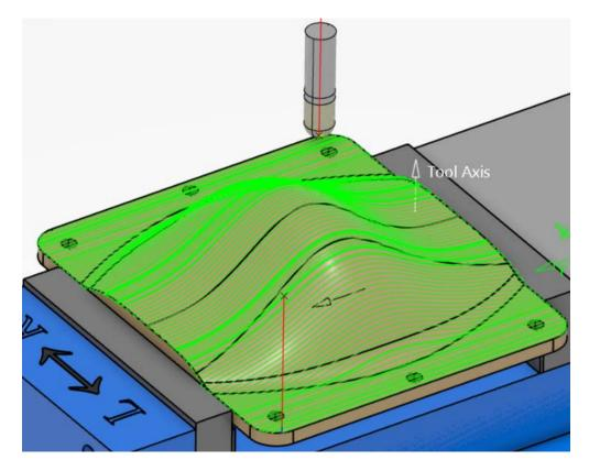
Under the *Axial* tab, set the *Number of levels* to 3, with a *Maximum cut depth* at 0.125in. This will indicate that you wish to have three sets of tool paths that are 0.125in apart. Take a look at the resulting tool paths, you will notice that it is a vertical offset from the bottom set of tool paths.
