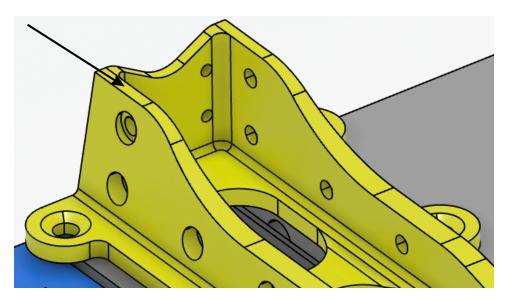
Simulate the operation. There is now a tool path at the same level as the imposed plane. If you look close, you should notice that the tool does not actually cut the top of the part.
