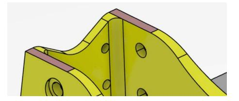
Select the *Reachable planes* button in the *Search* frame of the *Imposed planes search/view* window. This time, the list is reduced to the horizontal areas that can be reached by the tool. In this case, the 0.5in plane was removed. If other non-reachable planes existed, they would have been removed as well.
