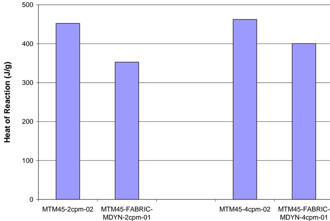
Lower total heat of reaction is measured for the fabric compared to the uni prepreg. The curing behaviour of the two forms, however, was found to be very similar. The error in the total HR of the fabric results in conservative estimation of exothermic events.
