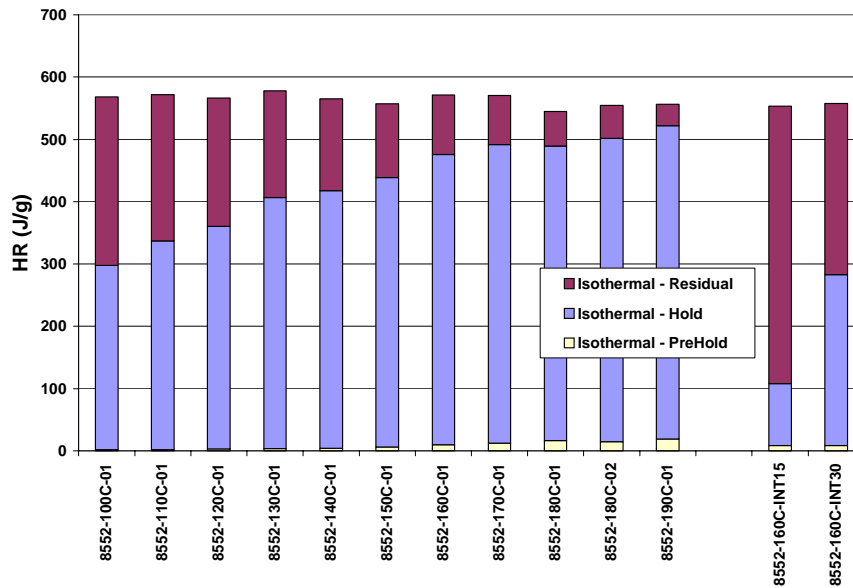
Figure 4. Heat of reaction calculated from the isothermal DSC tests.
