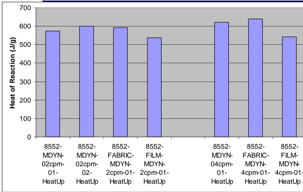
Lower total heat of reaction is measured for the film compared to the neat resin. Considering the similarities between the responses of neat resin and film up to 220C, the model (developed based on neat resin) is considered valid for resin film. The error in the total HR of the film results in conservative estimation of exothermic events.
