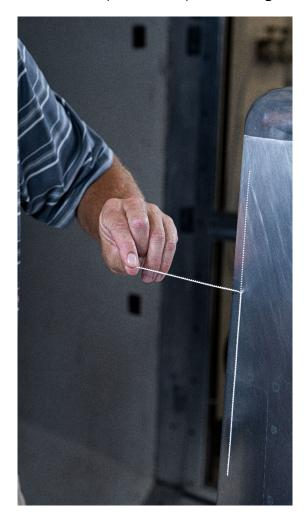
Step 8: Proceed with wind tunnel test. Monitor dot adhesion during model changes, etc. and replace as necessary.
