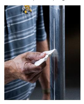
Step 6: Using sharp tool or fingernail, begin to lift one side of vinyl tape off model. Pro tip: when pulling tape, pull over the dot to help break adhesive between transition dot and rest of tape. You may have to experiment a bit with your application to find the best way to do this.
