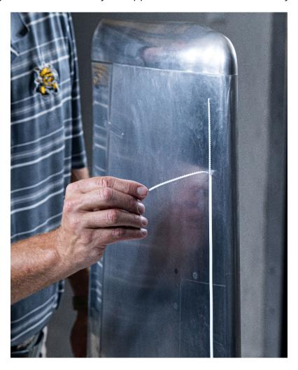
Step 7: Repeat for the other side of the vinyl tape. Only the transition dots should remain on the model. Using an X-Acto knife or similar, replace or reposition rogue dots as necessary.
