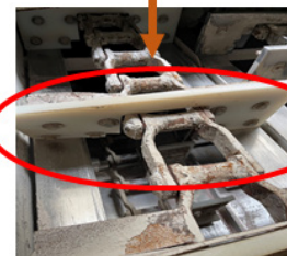
NO Warpage on Shocker Flights
