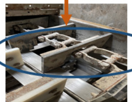
NO Warpage on Shocker Flights
