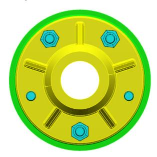
Delete the two nut instances that were added previously and delete the assembly pattern in the specification tree. Notice the patterned bolts are automatically removed as well.
