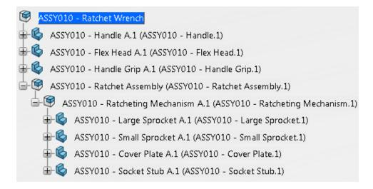
The Flex Head part should be part of the Ratchet Assembly. It will be added to the new subassembly.
