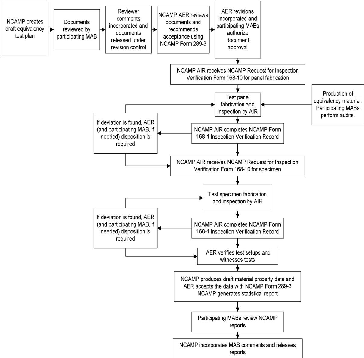
Figure 3. Flowchart of Equivalency Process for Part Fabricators
