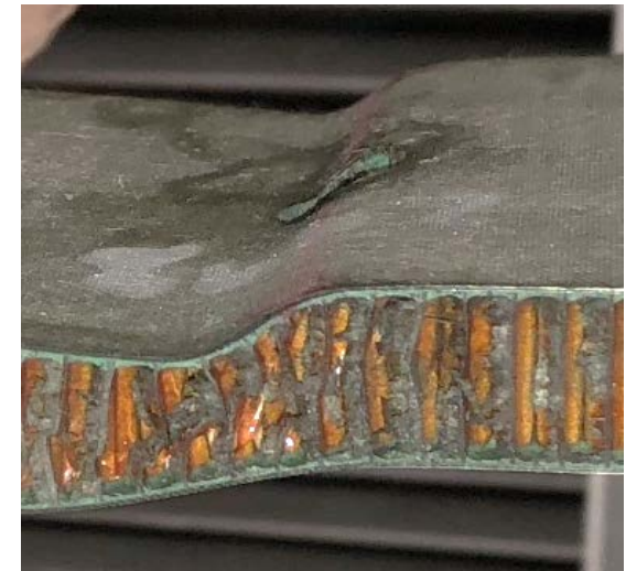
Sandwich Open-Hole Shear Failure
