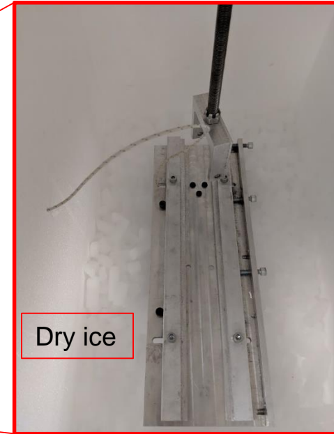
UW SCB test fixture immersed in a bed of dry ice
