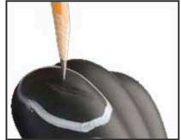
Grooves worn due to rope burns or heat exposure
