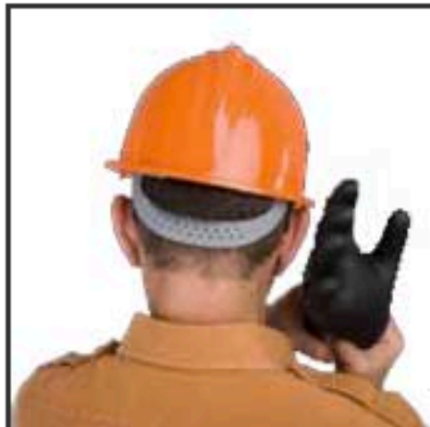
6. Hold close to ear, squeeze to add pressure, listen and feel for pinhole leaks
