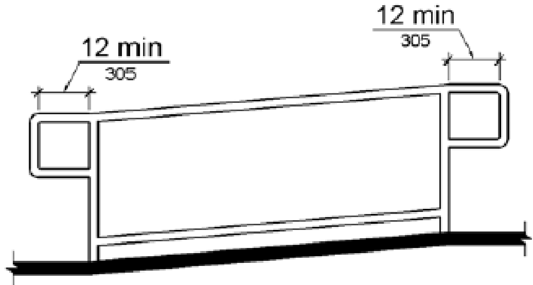
Figure 505.10.1 Top and Bottom Handrail Extension at Ramps
